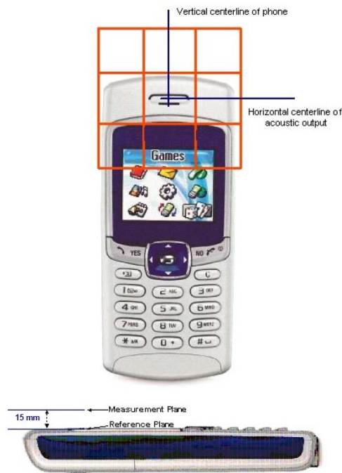
Figure 5.6-1: WD reference plane for RF emission measurement
