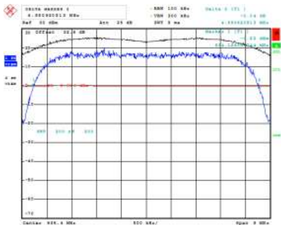
Figure 2-20a: -26 dBc Bandwidth, Band V Middle Channel
