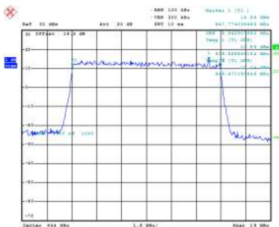
Figure 3-46a: Occupied Bandwidth, Band 5 Mid Channel, 20MHz BW (RB= 50) 16-QAM
