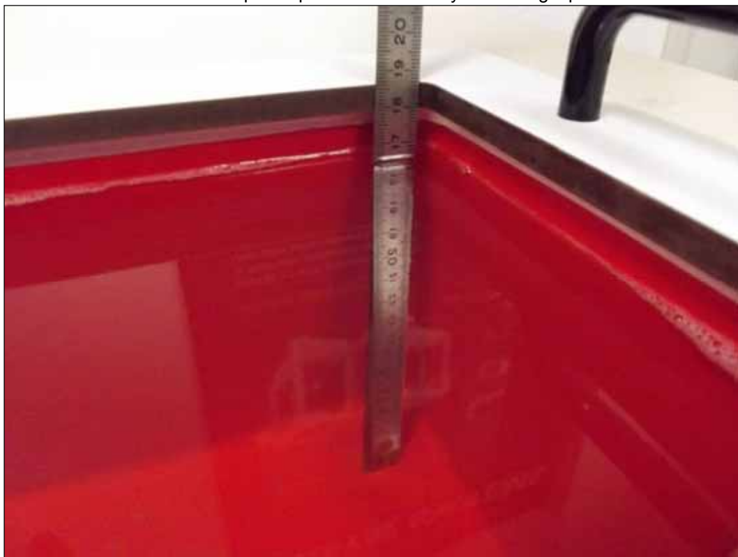
Photo 8: Liquid depth 1900 MHz body simulating liquid
