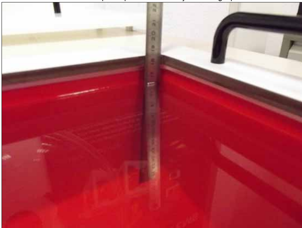
Photo 4: Liquid depth 850 MHz body simulating liquid
