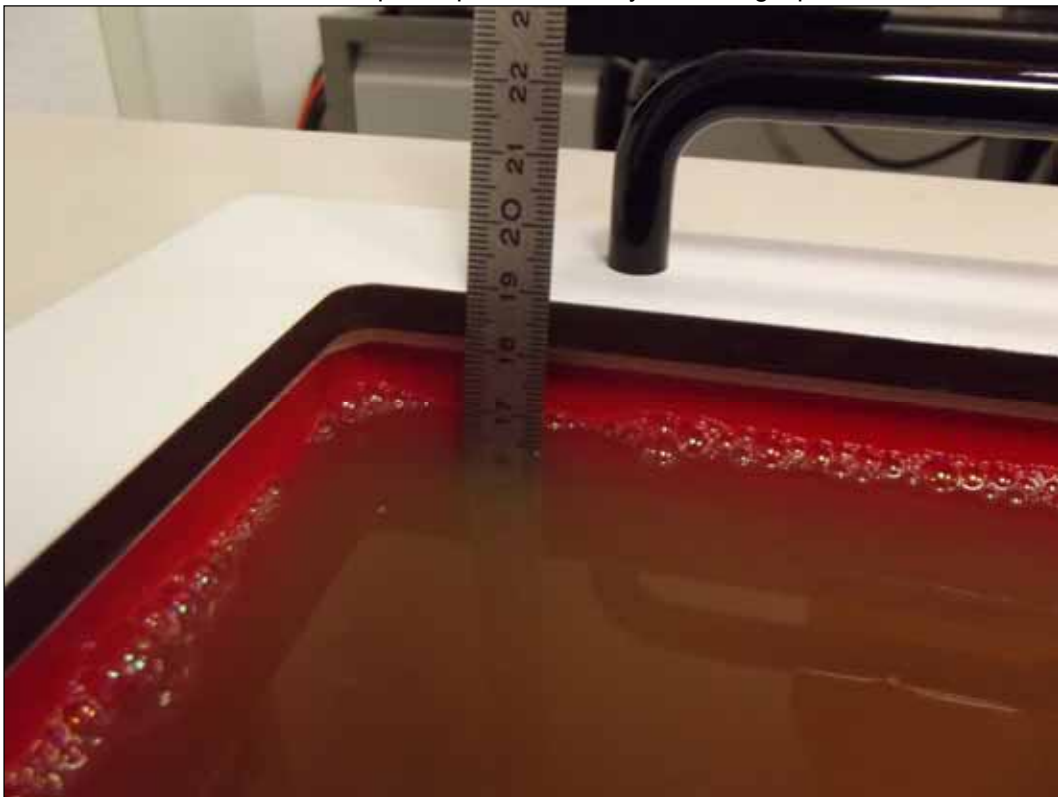
Photo 12: Liquid depth 5 GHz body simulating liquid
