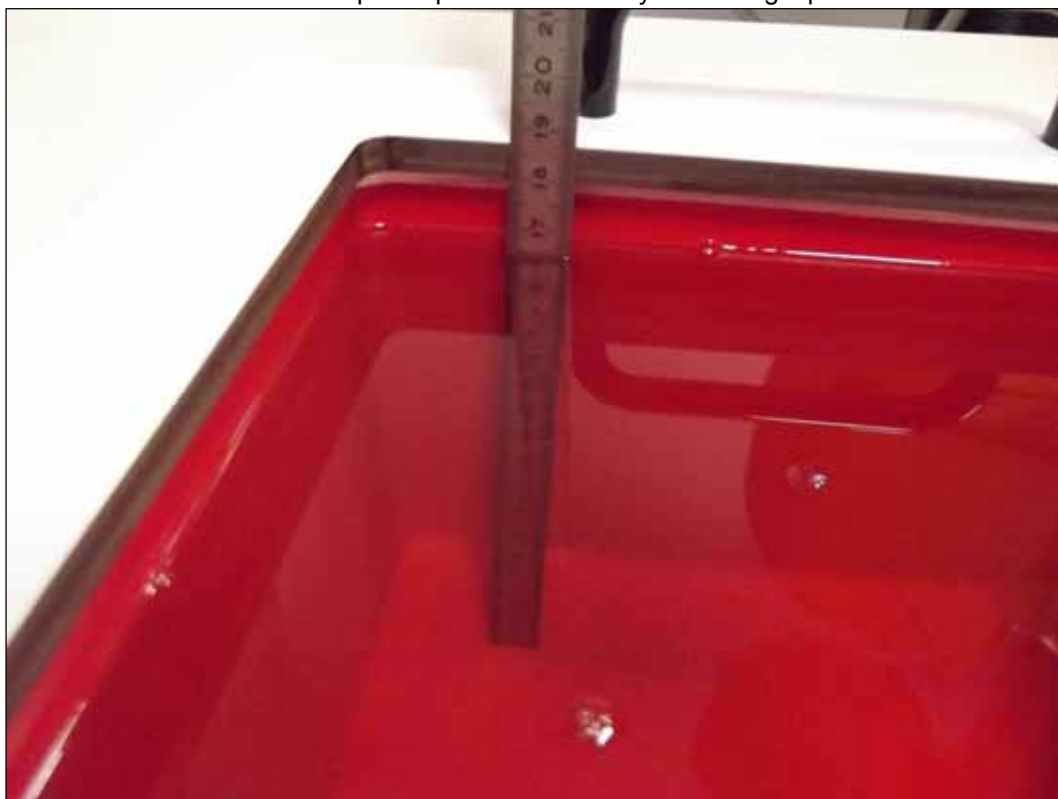
Photo 2: Liquid depth 750 MHz body simulating liquid
