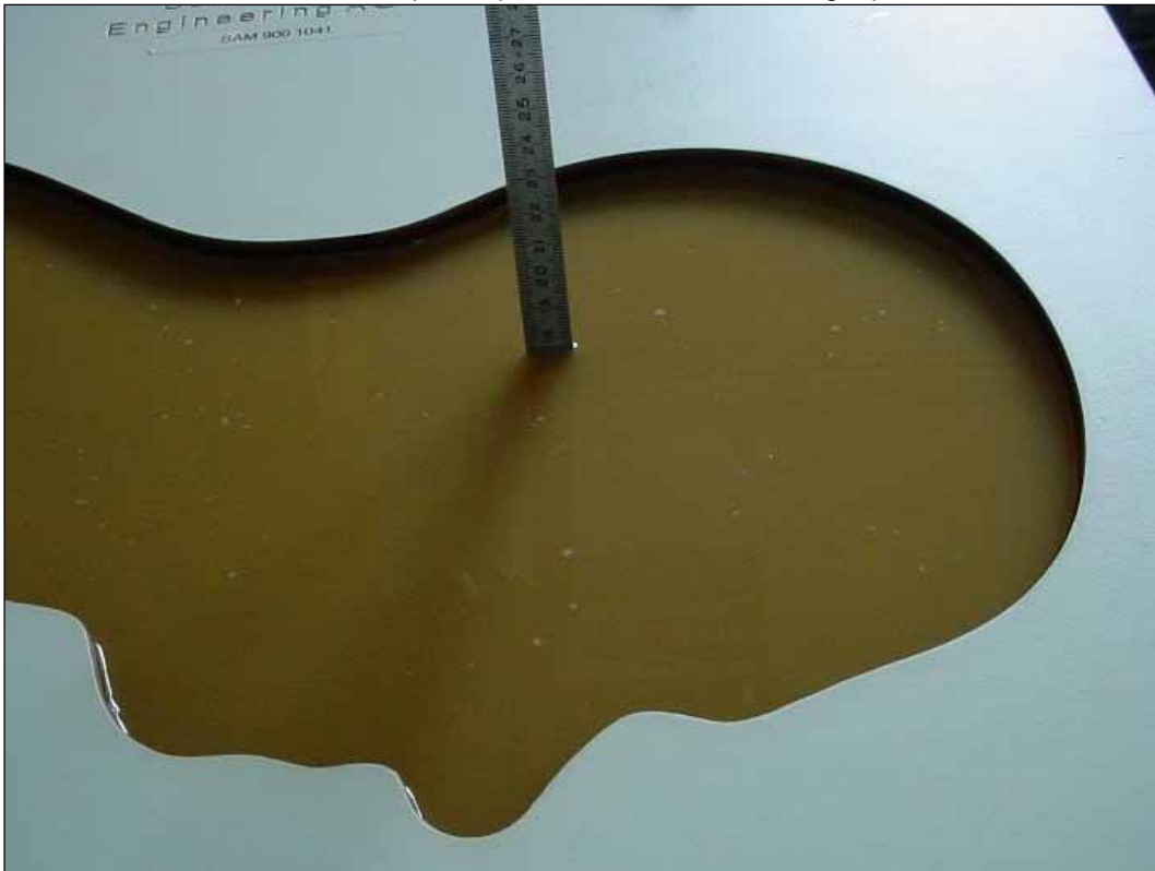
Photo 12: Liquid depth 5 GHz body simulating liquid
