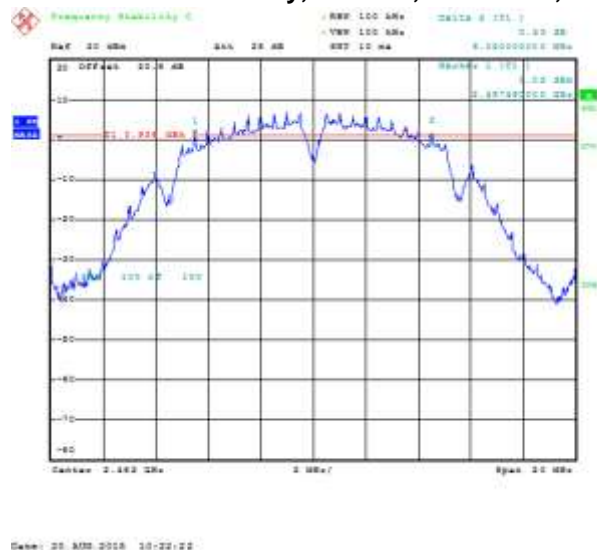
Figure 6-16: 6 dB Bandwidth Secondary, 802.11n, Channel 1, MCS 0
