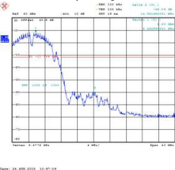
Figure 6-22: Band Edge Compliance Primary, 802.11g, Channel 11, 6 Mbps
