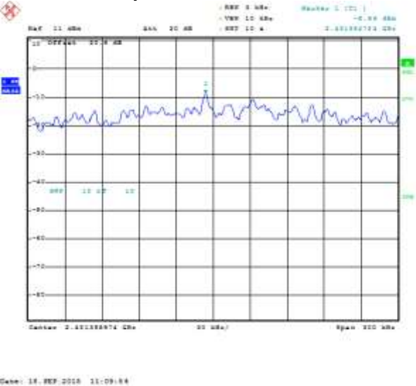
Figure 6-29: Peak Power Spectral Density SISO Primary, 802.11g, Channel 6, 6 Mbps
