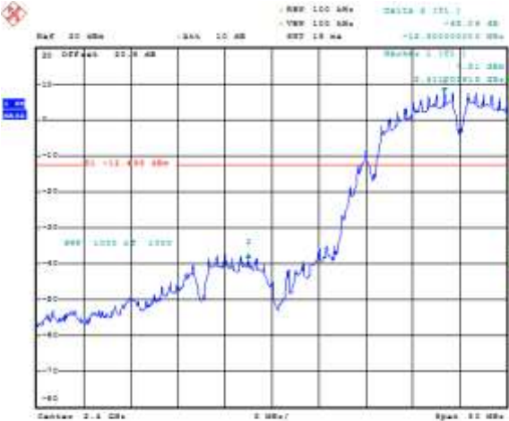
Figure 6-19: Band Edge Compliance Secondary, 802.11b, Channel 1, 1 Mbps
