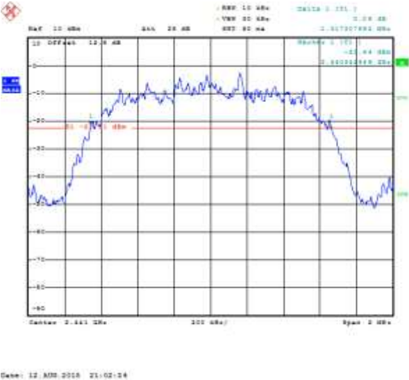
Figure 5-5: 20 dB Bandwidth Single freq. CH 39 Static PBRS, 2-DH5
