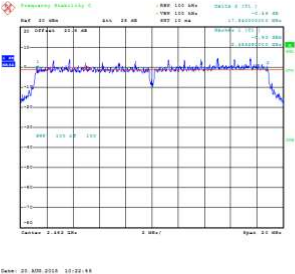
Figure 6-18: 6 dB Bandwidth Secondary, 802.11n, Channel 11, MCS 0
