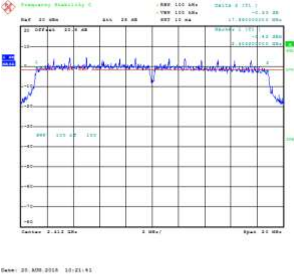
Figure 6-12: 6 dB Bandwidth Secondary, 802.11b, Channel 11, 1 Mbps
