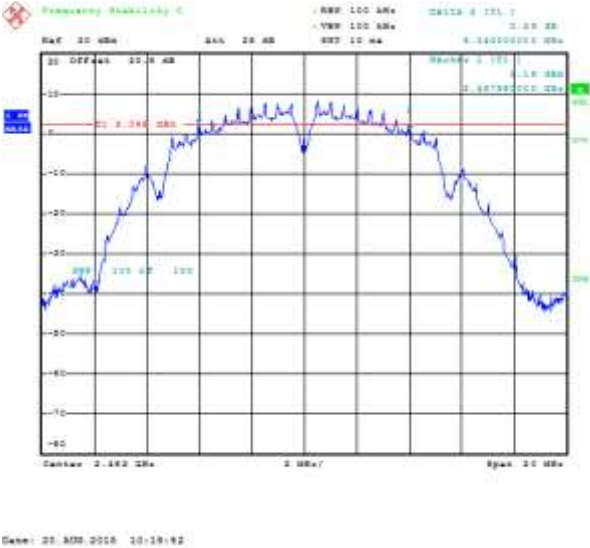
Figure 6-7: 6 dB Bandwidth Primary, 802.11n, Channel 1, MCS 0
