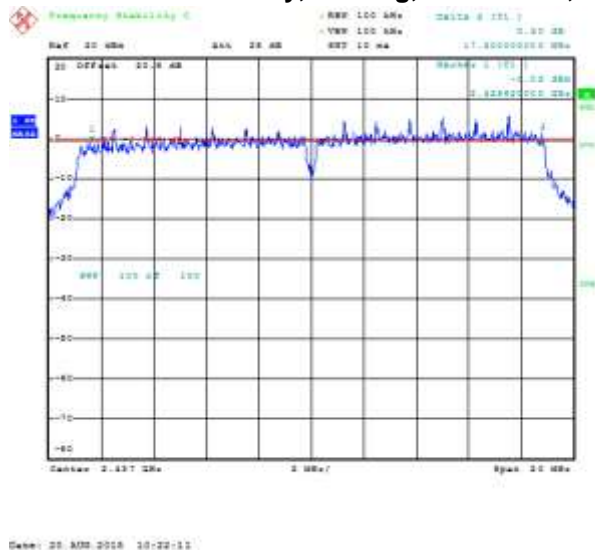
Figure 6-15: 6 dB Bandwidth Secondary, 802.11g, Channel 11, 6 Mbps
