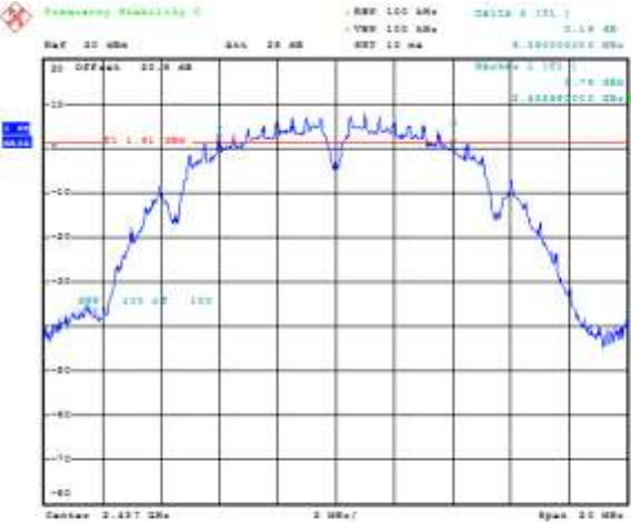
Figure 6-4: 6 dB Bandwidth Primary, 802.11g, Channel 1, 6 Mbps
