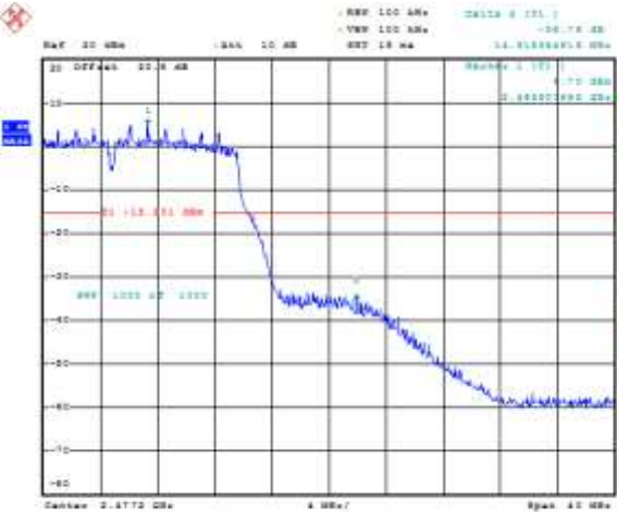
Figure 6-24: Band Edge Compliance Primary, 802.11n, Channel 11, MCS 0
