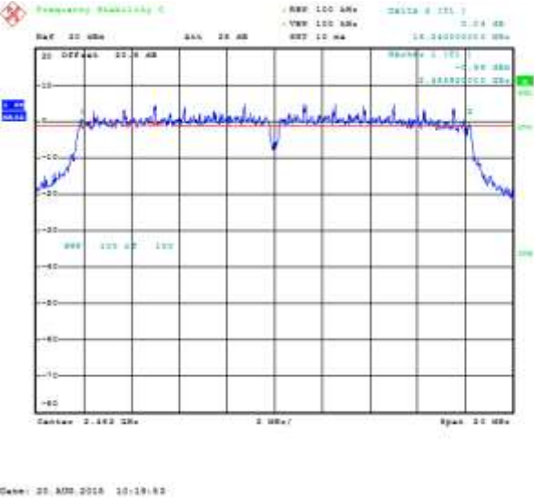
Figure 6-8: 6 dB Bandwidth Primary, 802.11n, Channel 6, MCS 0
