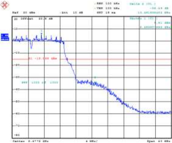
Figure 6-23: Band Edge Compliance Primary, 802.11n, Channel 1, MCS 0
