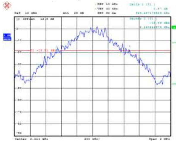
Figure 5-2: 20 dB Bandwidth Single freq. CH 39 Static PBRS, DH5
