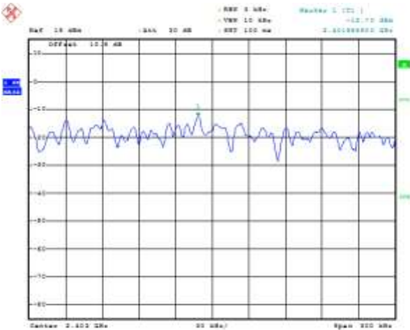
Figure 5-55: Peak Power Spectral Density LE, Channel 0
