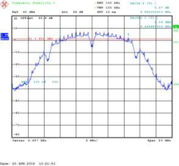
Figure 6-13: 6 dB Bandwidth Secondary, 802.11g, Channel 1, 6 Mbps
