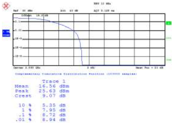
Figure 11-68a: Band 41 Mid Channel PAR, 5MHz BW, RB=10
