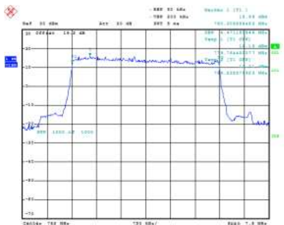
Figure 9-16a: Occupied Bandwidth, Band 5 Middle Channel, 5MHz BW, RB=50
