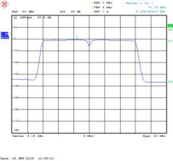
Figure 7-110: Peak Power Spectral Density SISO Secondary, 802.11n, Channel 36, MCS 0
