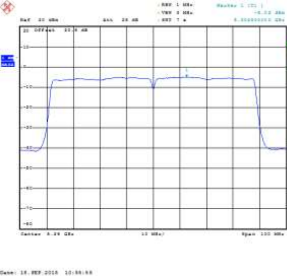
Figure 8-101: Peak Power Spectral Density SISO Secondary, 802.11ac, Channel 58, MCS0 Mbps
