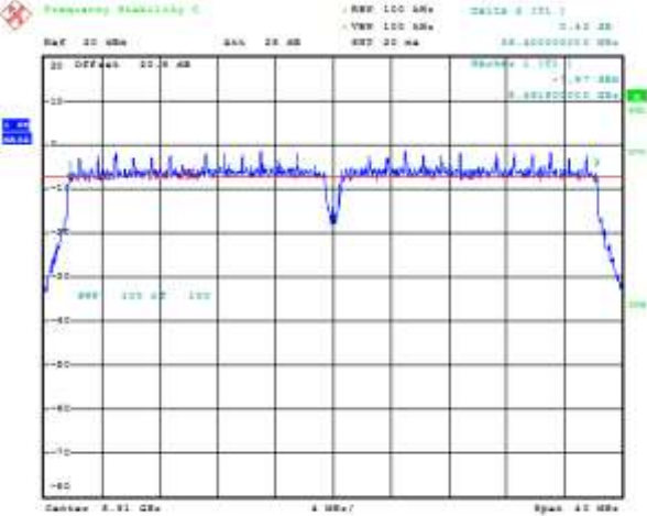
Figure 8-18: 6 dB Bandwidth Secondary, 802.11ac, Channel 100, 6 Mbps
