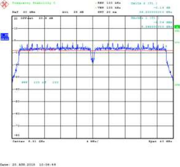
Figure 8-12: 6 dB Bandwidth Primary, 802.11ac, Channel 64, MCS0 Mbps
