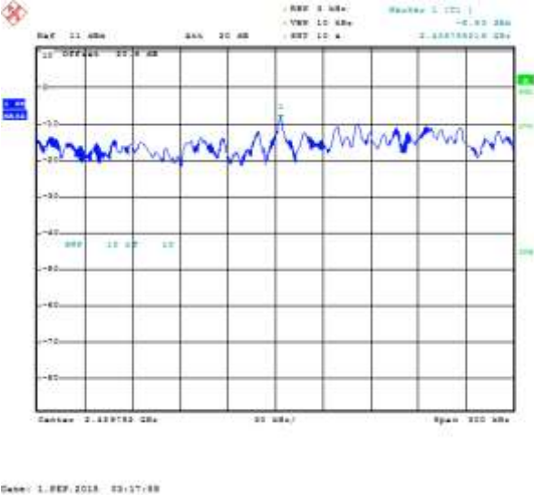
Figure 6-56: Peak Power Spectral Density MIMO Secondary, 802.11g, Channel 6, 6 Mbps
