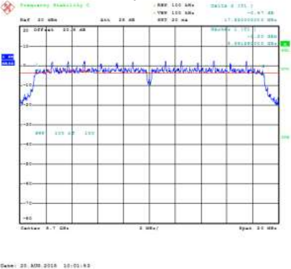
Figure 8-9: 6 dB Bandwidth Secondary, 802.11ac, Channel 140, MCS0 Mbps
