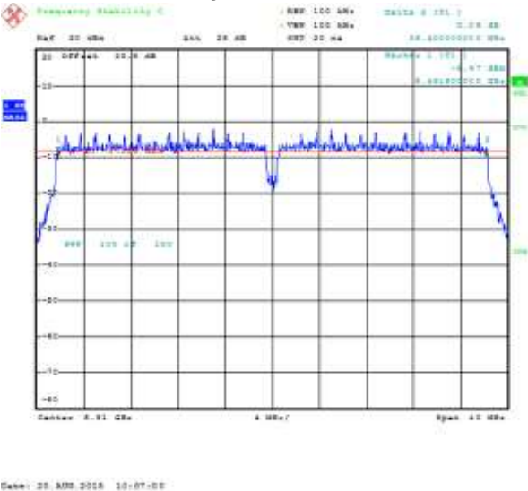
Figure 8-13: 6 dB Bandwidth Primary, 802.11ac, Channel 100, 6 Mbps
