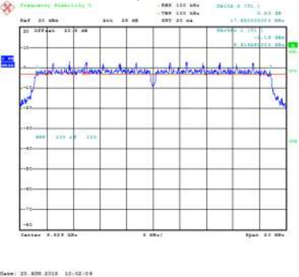
Figure 8-10: 6 dB Bandwidth Secondary, 802.11ac, Channel 149, MCS0 Mbps
