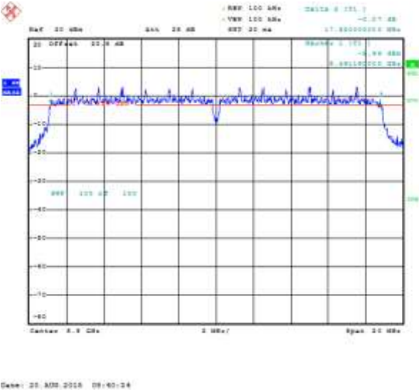
Figure 7-15: 6 dB Bandwidth Primary, 802.11n, Channel 100, MCS 0
