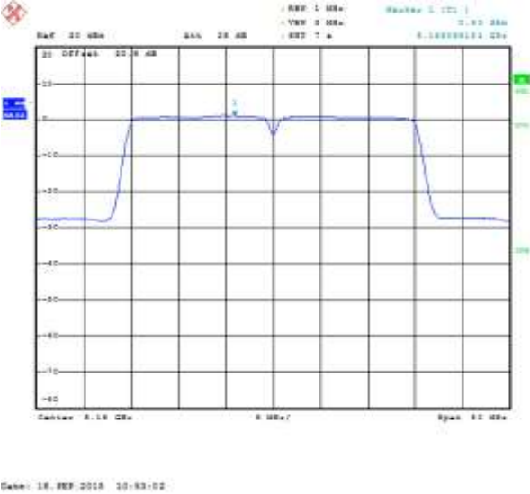
Figure 8-83: Peak Power Spectral Density SISO Secondary, 802.11ac, Channel 38, MCS0 Mbps
