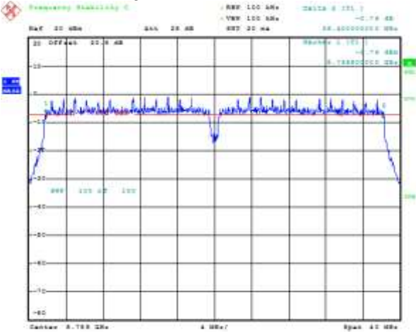
Figure 8-15: 6 dB Bandwidth Primary, 802.11ac, Channel 149, MCS0 Mbps
