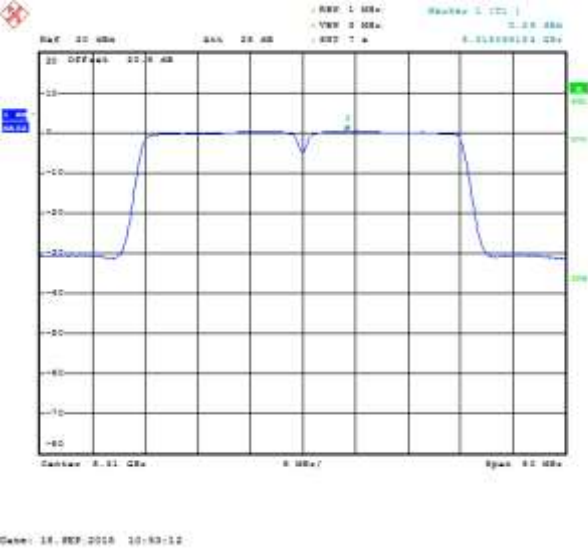
Figure 8-84: Peak Power Spectral Density SISO Secondary, 802.11ac, Channel 62, MCS0 Mbps
