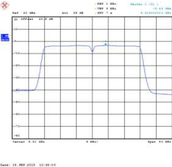
Figure 7-107: Peak Power Spectral Density SISO Primary, 802.11n, Channel 64, MCS 0
