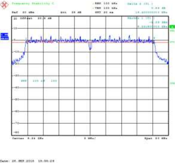
Figure 7-8: 6 dB Bandwidth Secondary, 802.11a, Channel 48, 6 Mbps
