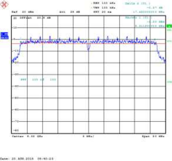
Figure 7-14: 6 dB Bandwidth Primary, 802.11n, Channel 64, MCS 0
