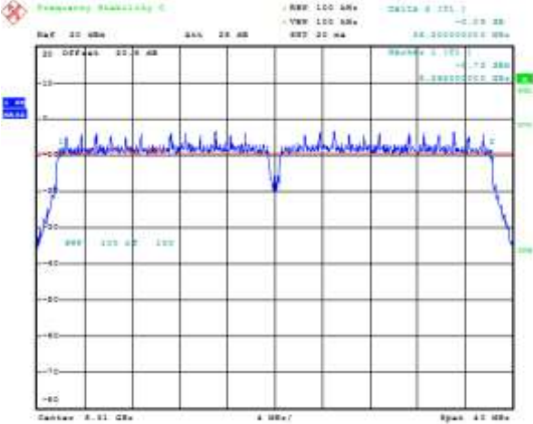
Figure 8-17: 6 dB Bandwidth Secondary, 802.11ac, Channel 64, 6 Mbps
