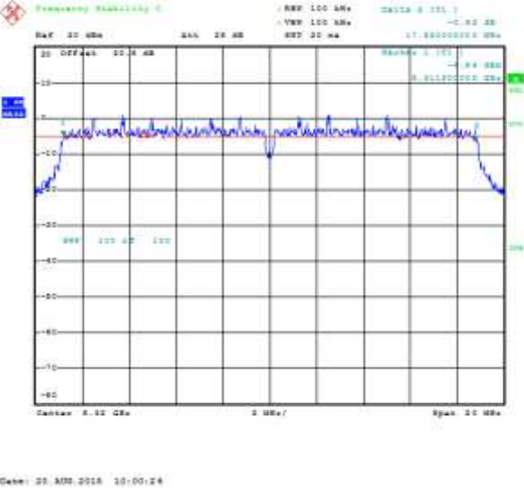
Figure 8-2: 6 dB Bandwidth Primary, 802.11ac, Channel 64, MCS0 Mbps
