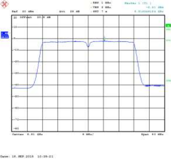
Figure 7-112: Peak Power Spectral Density SISO Secondary, 802.11n, Channel 100, MCS 0
