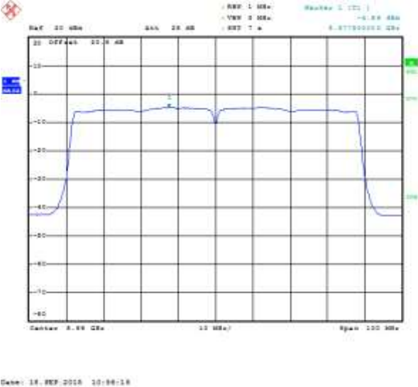
Figure 8-104: Peak Power Spectral Density SISO Secondary, 802.11ac, Channel 155, MCS0 Mbps
