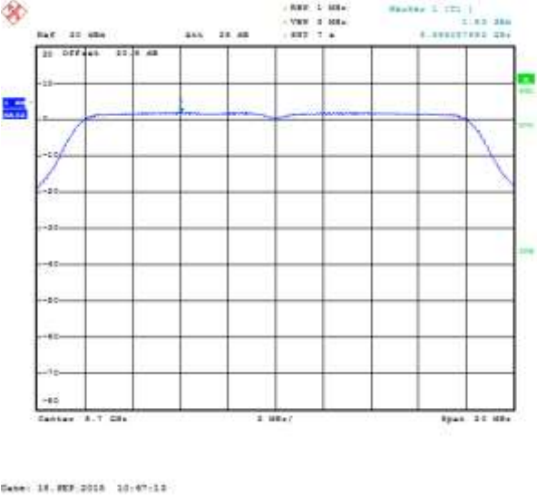
Figure 7-76: Peak Power Spectral Density SISO Secondary, 802.11a, Channel 140, 6 Mbps
