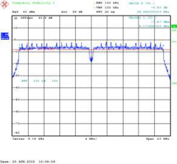
Figure 8-11: 6 dB Bandwidth Primary, 802.11ac, Channel 36, MCS0 Mbps
