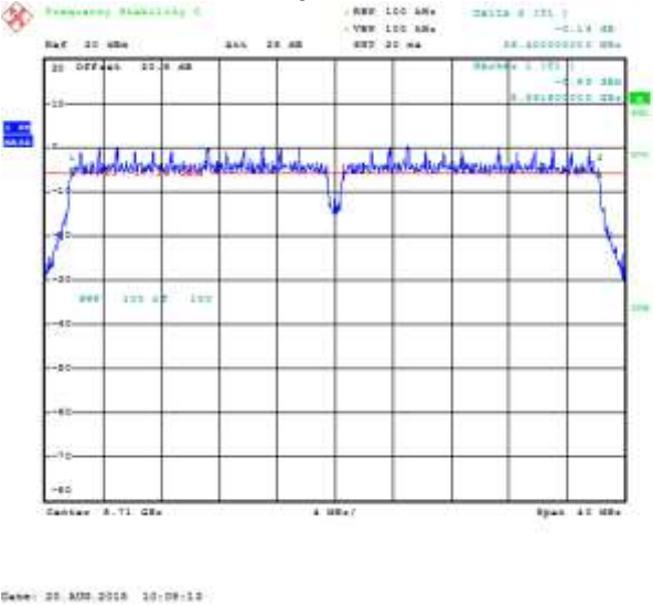
Figure 8-19: 6 dB Bandwidth Secondary, 802.11ac, Channel 140, MCS0 Mbps
