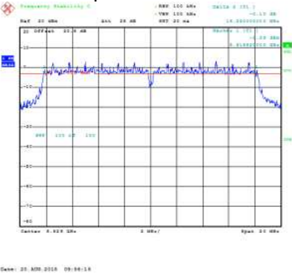
Figure 7-12: 6 dB Bandwidth Secondary, 802.11a, Channel 165, 6 Mbps
