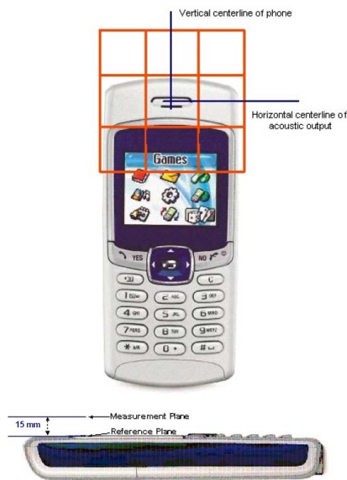
Figure 5.6-1: WD reference plane for RF emission measurement
