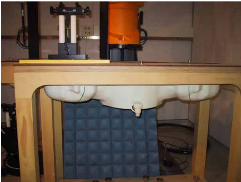
Figure 10.1-1 DASy5 system with absorbing material
