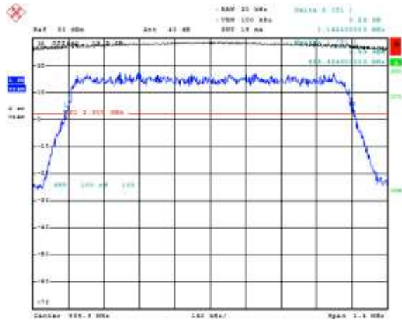
Figure 4-35a: -26 dBc Bandwidth, Band 5 Middle Channel, 1.4MHz BW, RB=6
