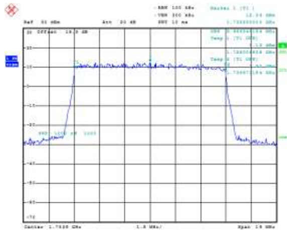
Figure 5-23a: Occupied Bandwidth, Band Middle Channel, 10MHz BW, RB=50
