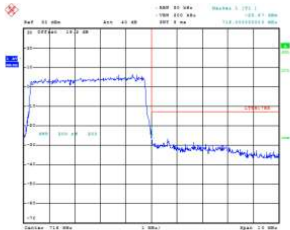
Figure 6-30a: Band 17 High Channel Mask, 5MHz BW, RB=25
