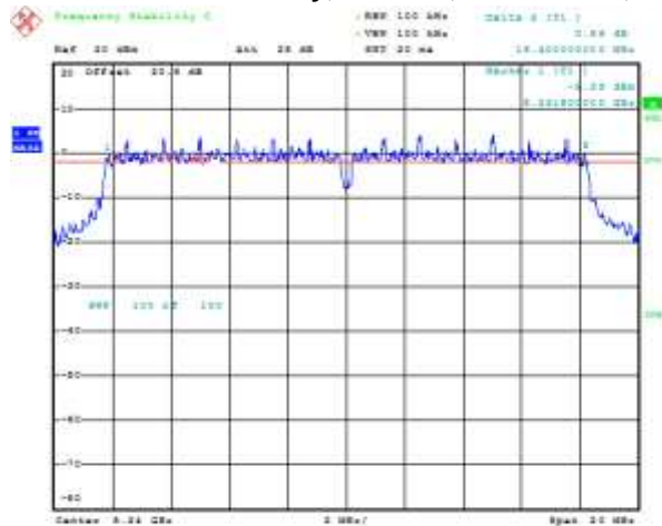
Figure 7-8: 6 dB Bandwidth Secondary, 802.11a, Channel 48, 6 Mbps
