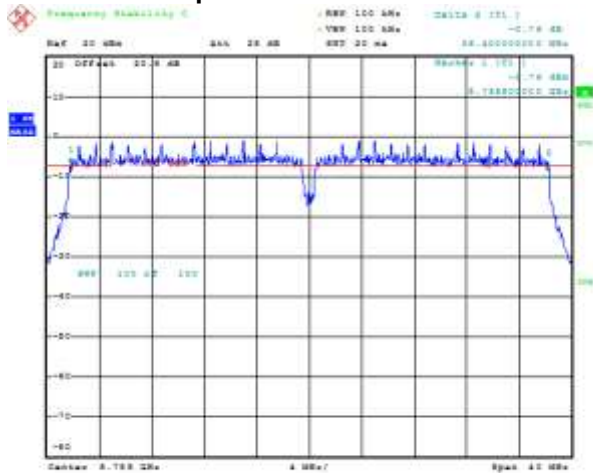
Figure 8-15: 6 dB Bandwidth Primary, 802.11ac, Channel 149, MCS0 Mbps
