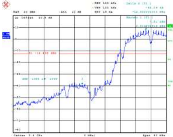
Figure 6-19: Band Edge Compliance Secondary, 802.11b, Channel 1, 1 Mbps
