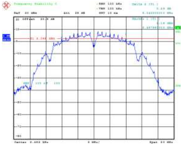
Figure 6-7: 6 dB Bandwidth Primary, 802.11n, Channel 1, MCS 0
