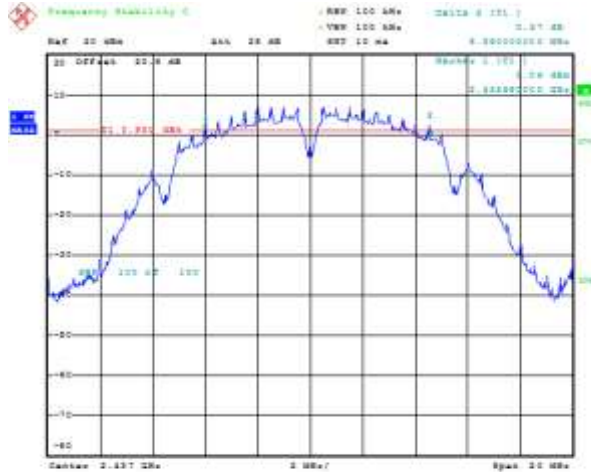
Figure 6-13: 6 dB Bandwidth Secondary, 802.11g, Channel 1, 6 Mbps
