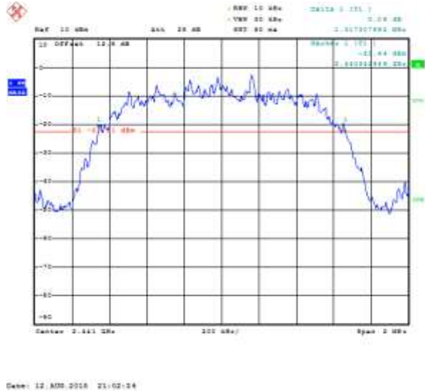
Figure 5-5: 20 dB Bandwidth Single freq. CH 39 Static PBRs, 2-DH5
