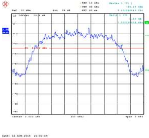
Figure 5-4: 20 dB Bandwidth Single freq. CH 0 Static PBRs, 2-DH5
