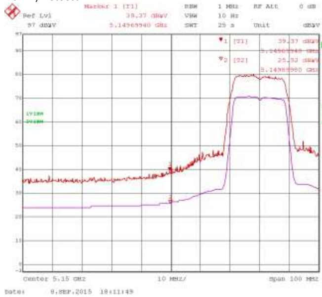
Figure 4-23: Band-Edge Compliance of RF Radiated Emission 802.11ac, Secondary, Ch. 64, 5320 MHz, Centre of Band-Edge: 5350 MHz Pol: V, Detector: PK
