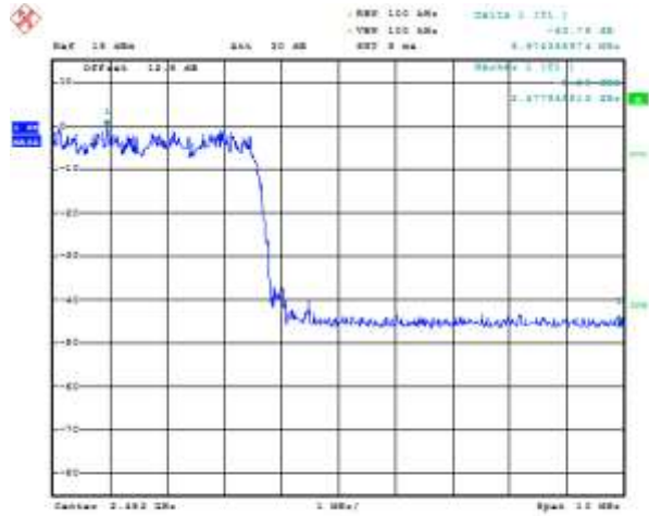
Figure 5-37: Band Edge Compliance Freq. Hopping, Static PBRS, 3-DH5
