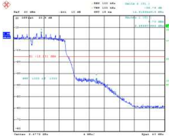
Figure 6-24: Band Edge Compliance Primary, 802.11n, Channel 11, MCS 0
