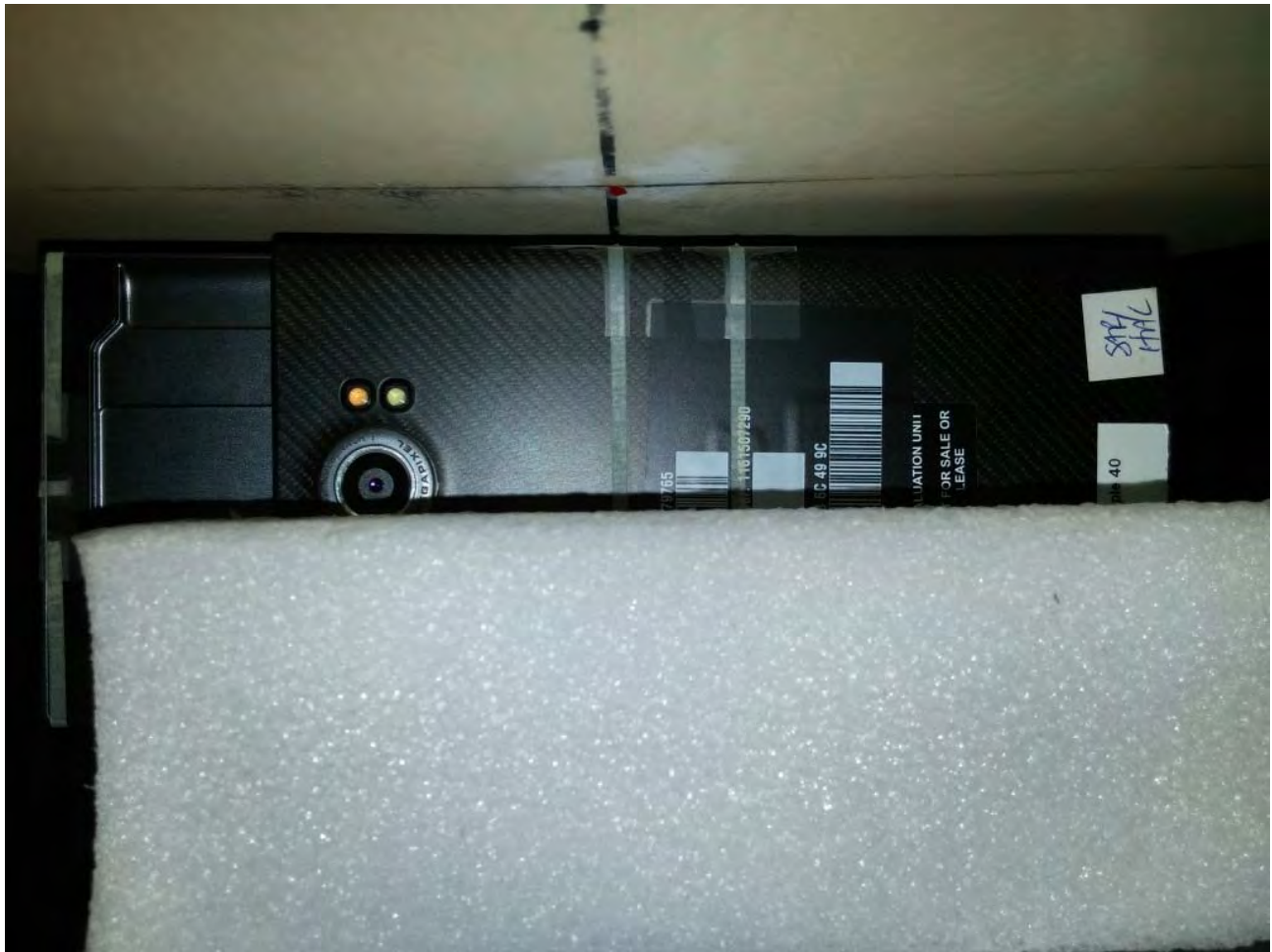
Figure E14. Hotspot configuration – Slider Open (No Holster, left side 10mm away)
