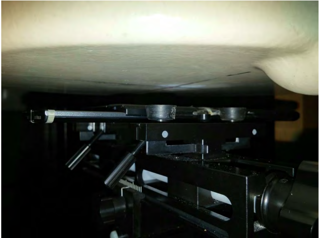
Figure E22. Body-worn configuration – Slider Open (No Holster, back side 15mm away)
