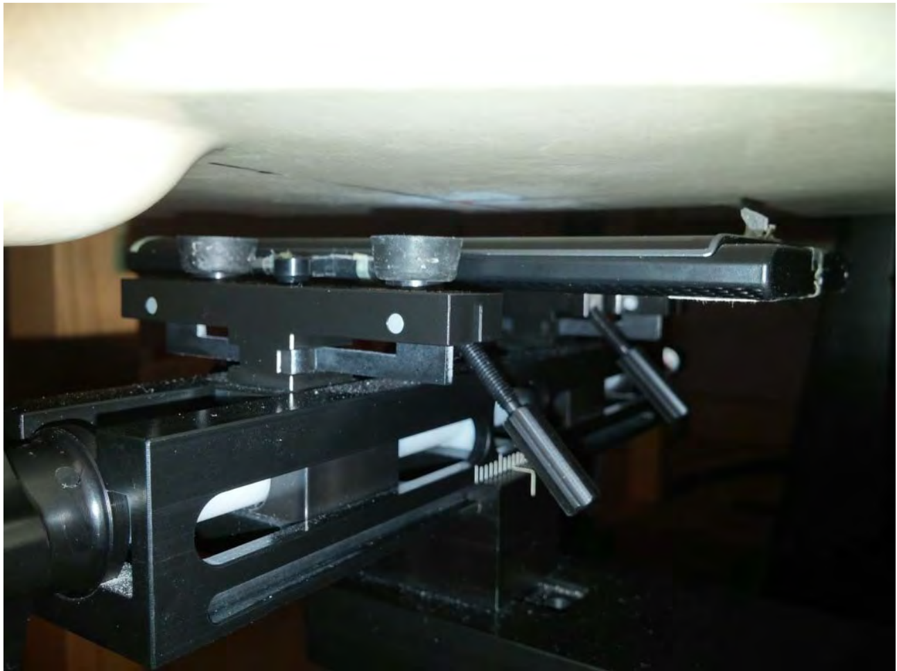
Figure E11. Hotspot configuration – Slider Closed (No Holster, front side 10mm away)
