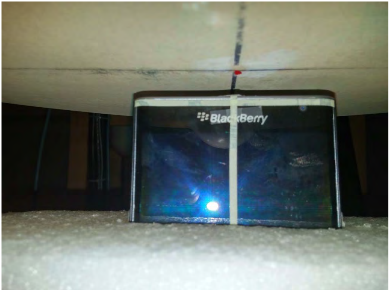
Figure E17. Hotspot configuration – Slider Closed (No Holster, top side 10mm away)
