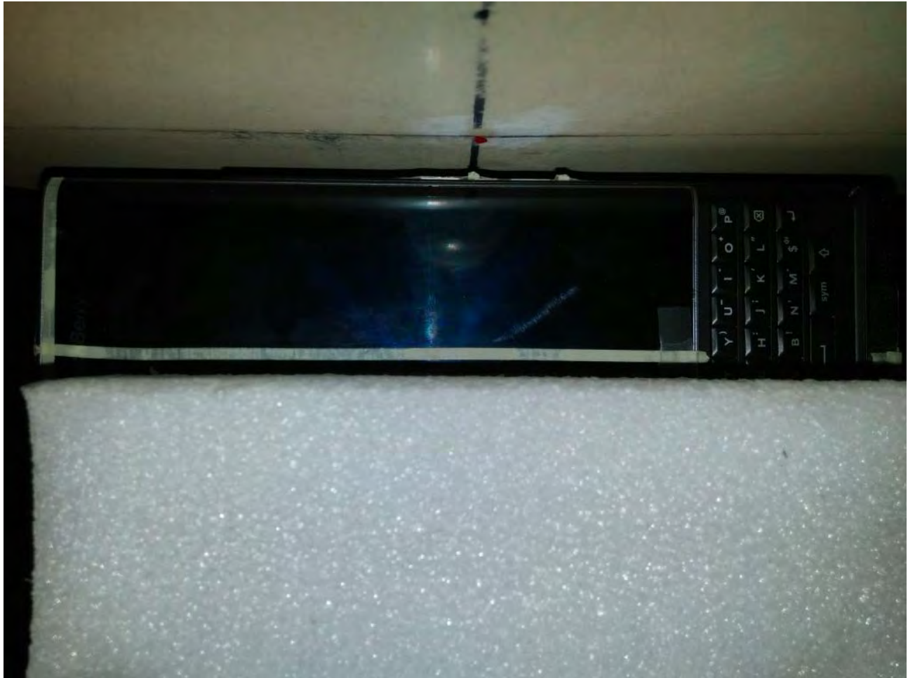
Figure E16. Hotspot configuration – Slider Open (No Holster, right side 10mm away)
