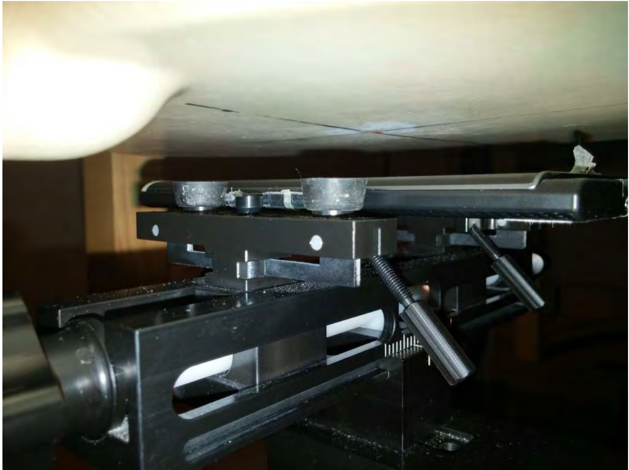
Figure E23. Body-worn configuration – Slider Closed (No Holster, front side 15mm away)
