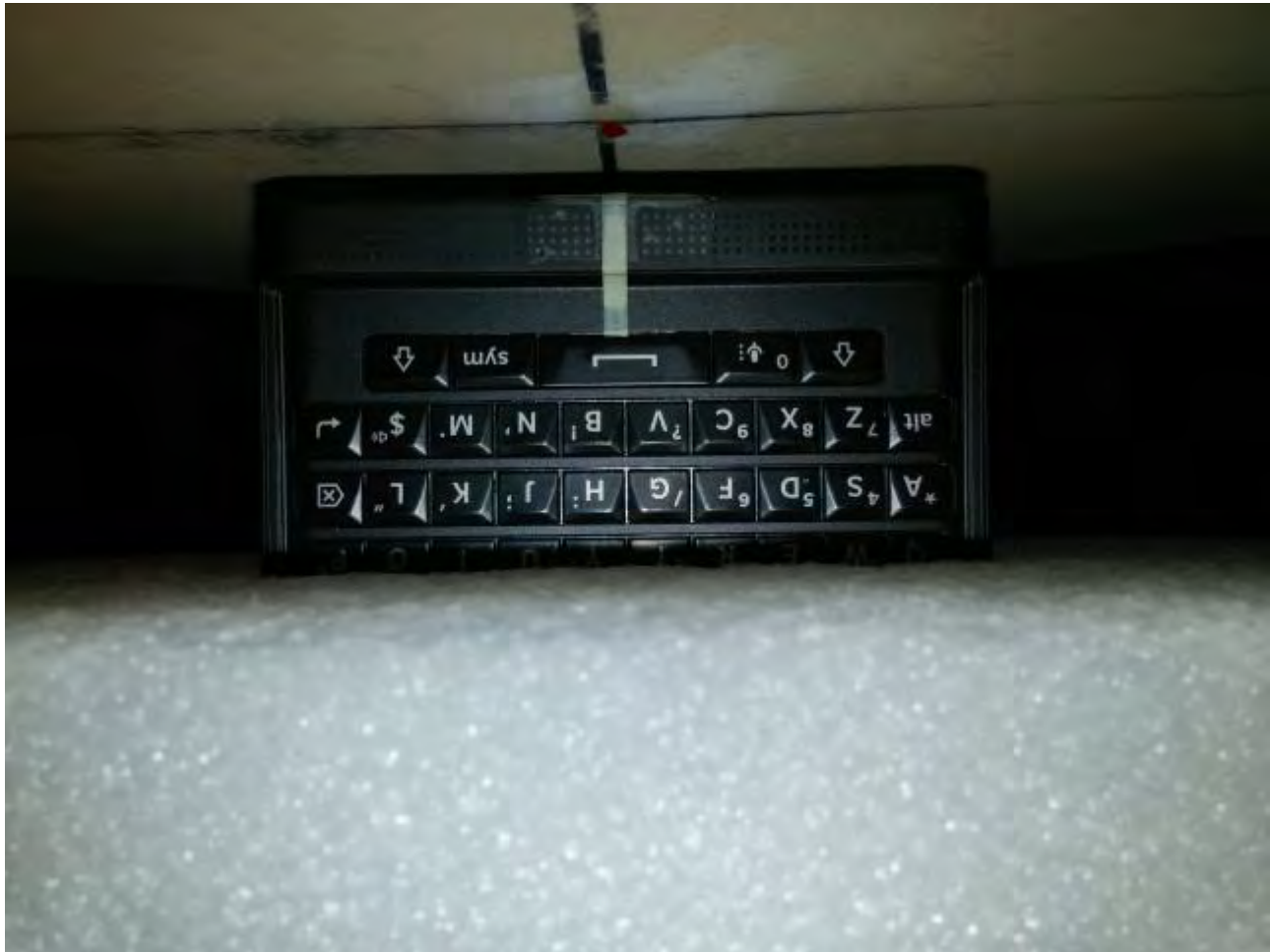
Figure E20. Hotspot configuration – Slider Open (No Holster, bottom side 10mm away)
