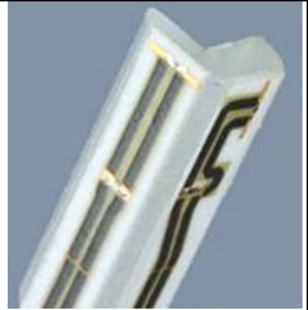
Fig 5.2 Photo of E-field Probe
