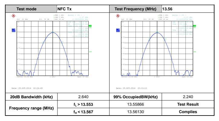
C.1 Test Result of 20dB Spectrum Bandwidth
