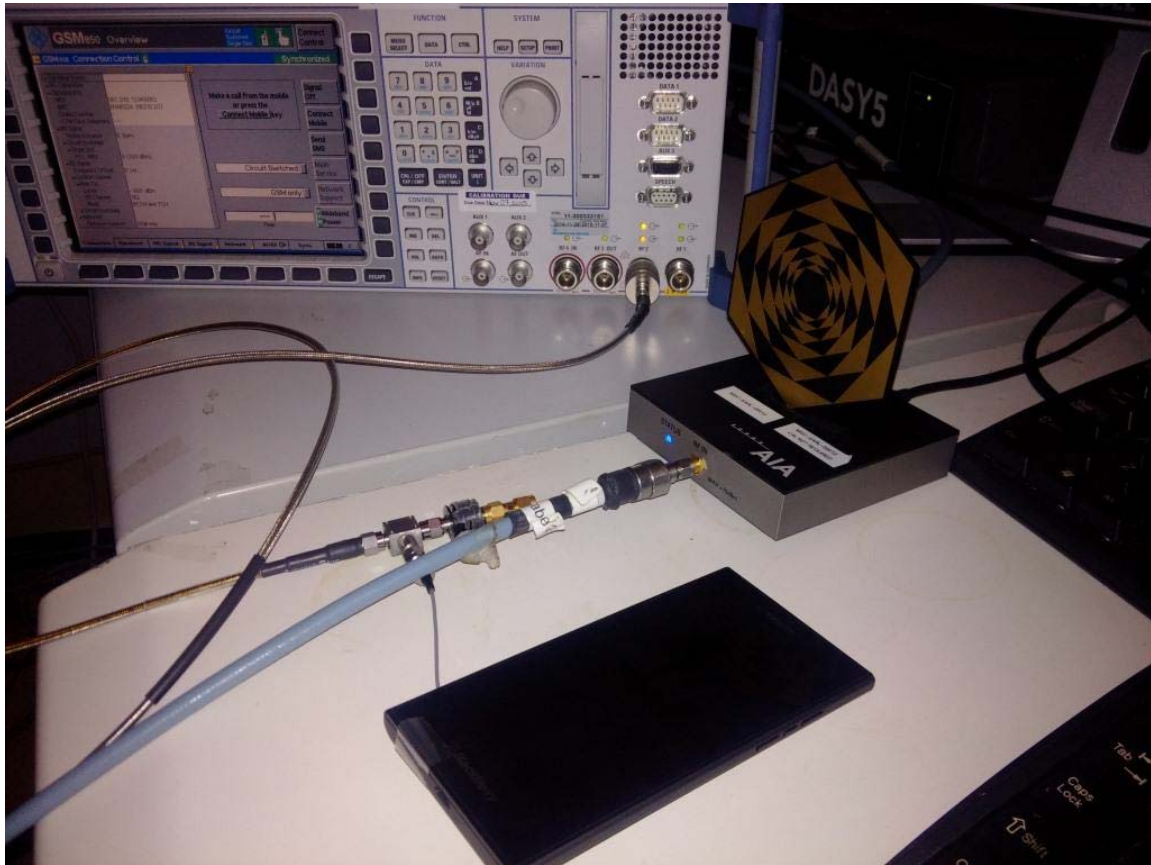
Figure C2 – MIF measurement setup
