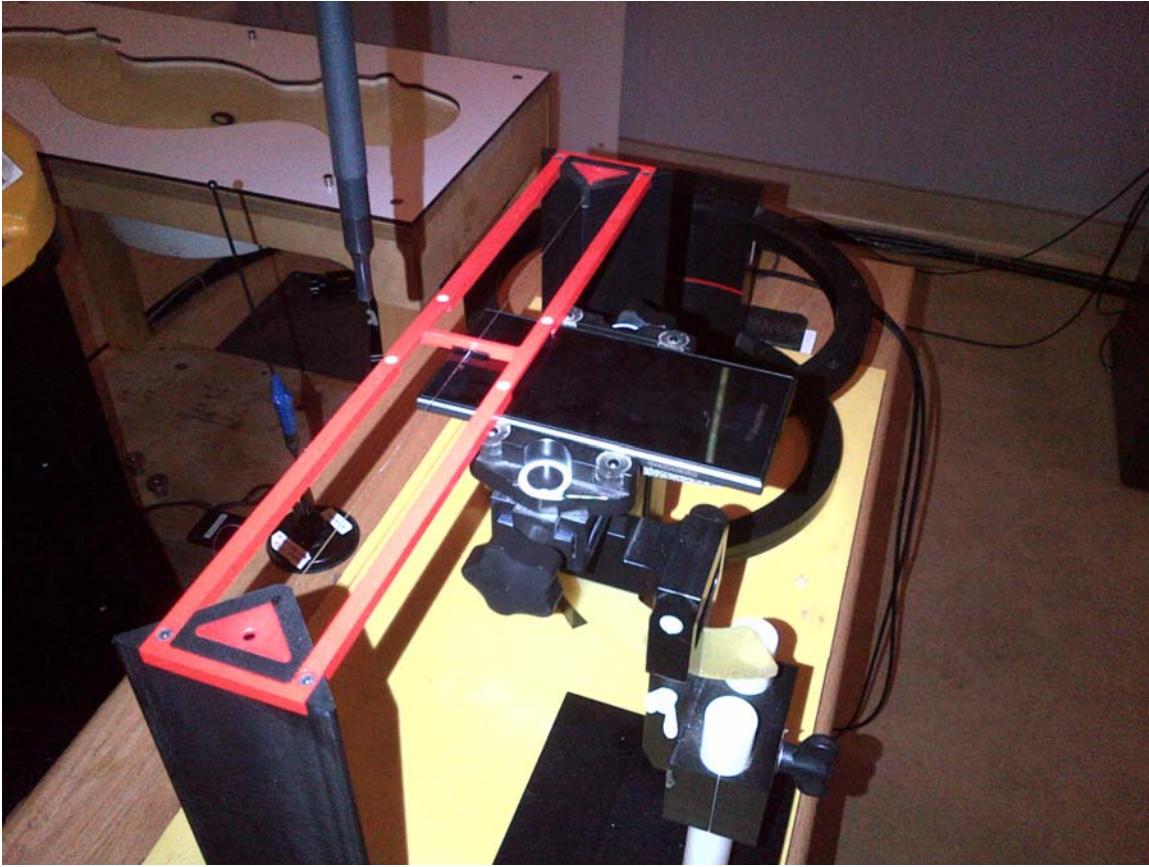
Figure C4 – HAC RF emissions test setup
