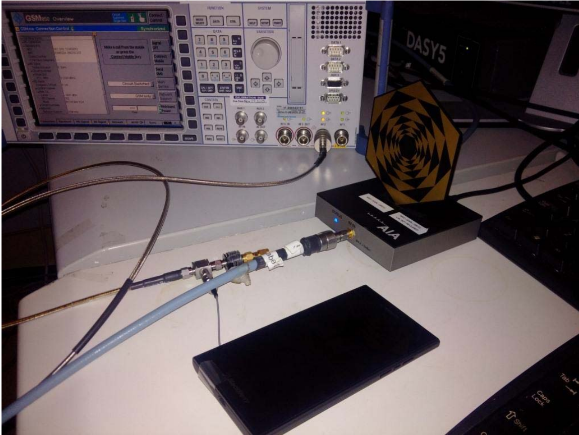
Figure C2 – MIF measurement setup
