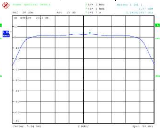
Figure 3-2: Peak Power Spectral Density 802.11a, Channel 48, 6 Mbps
