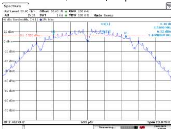
Figure 2-3: 6 dB Bandwidth 802.11b, Channel 11, 1 Mbps
