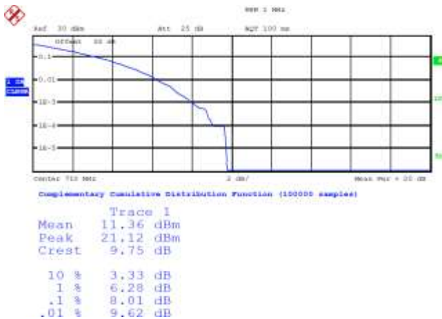
Figure 6-33a: Band 17 Mid Channel PAR, 10MHz BW, RB=25
