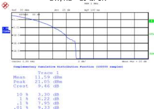
Figure 3-39a: Band 2, Mid Channel PAR, 10 MHz BW, RB = 25 QPSK
