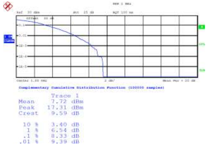
Figure 3-38a: Band 2, Mid Channel PAR, 20 MHz BW, RB = 100 16-QAM
