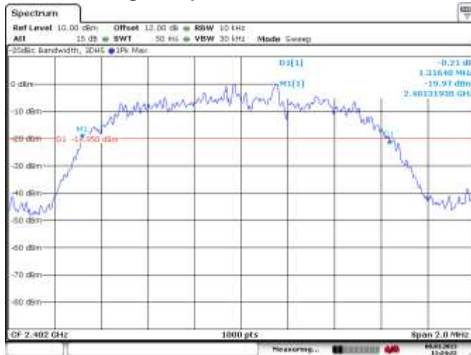
Figure 4-9: 20 dB Bandwidth Single freq., Static PBRs, 3-DH5
