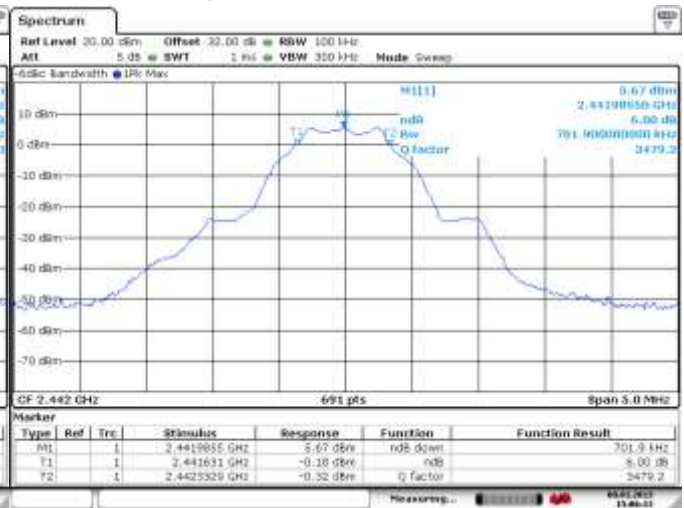
Figure 4-60: 6 dB Bandwidth LE, Channel 20
