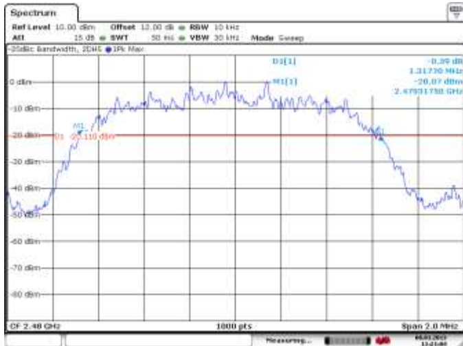
Figure 4-6: 20 dB Bandwidth Single freq., Static PBRs, 2-DH5
