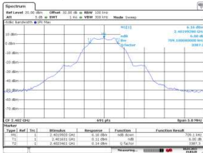
Figure 4-59: 6 dB Bandwidth LE, Channel 0
