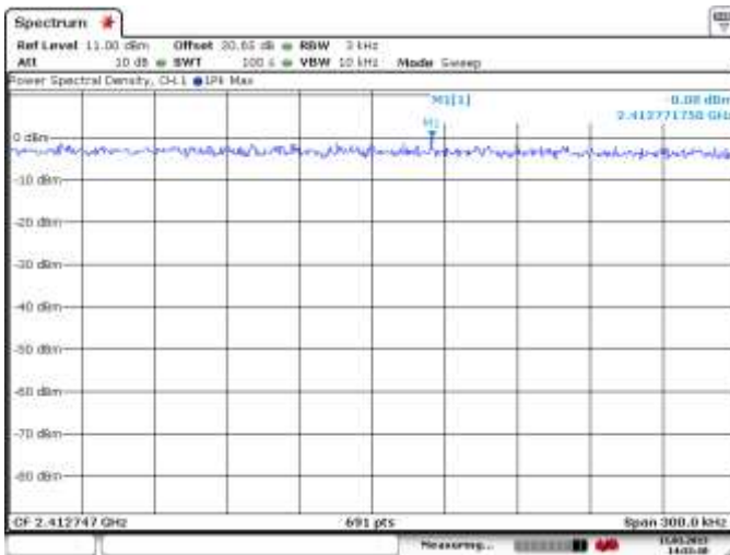
Figure 5-16: Peak Power Spectral Density 802.11b, Channel 1, 1 Mbps
