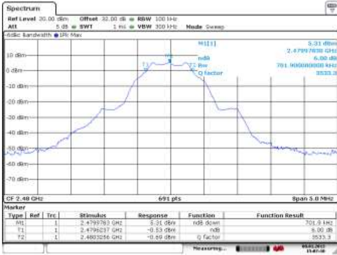
Figure 4-61: 6 dB Bandwidth LE, Channel 39
