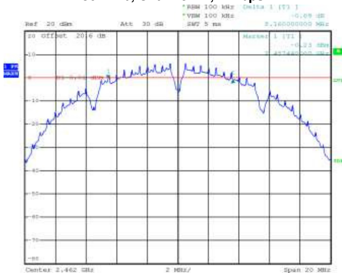
Figure 6-3: 6 dB Bandwidth 802.11b, Channel 11, 1 Mbps
