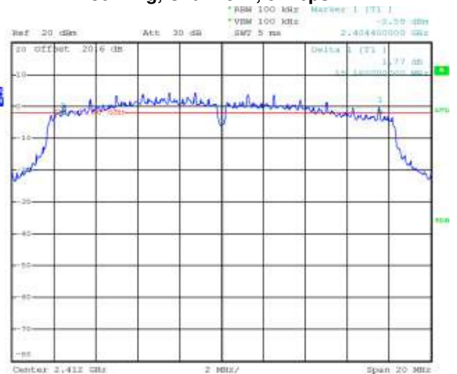
Figure 6-4: 6 dB Bandwidth 802.11g, Channel 1, 6 Mbps
