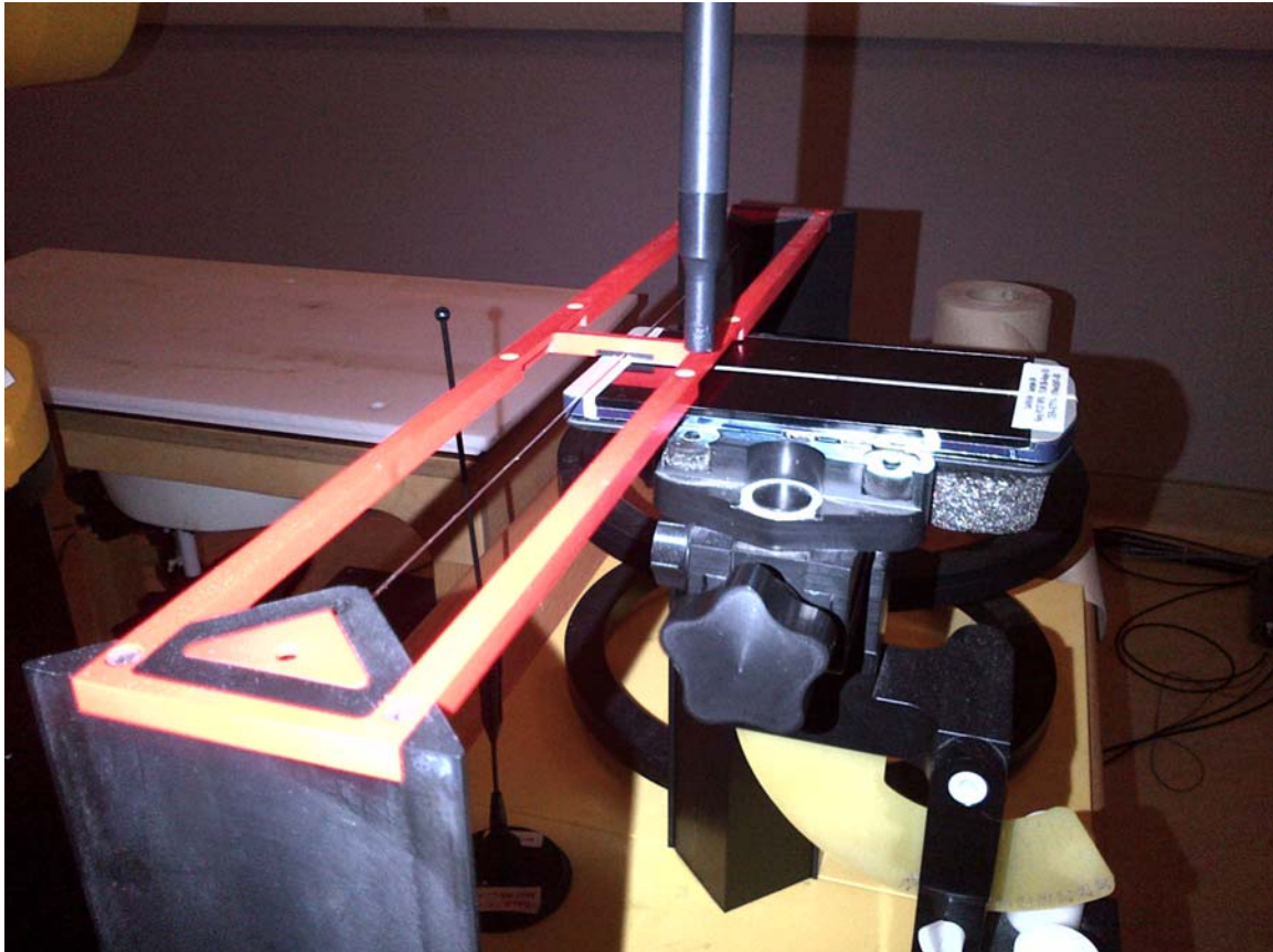
Figure C3 – HAC RF emission test setup
