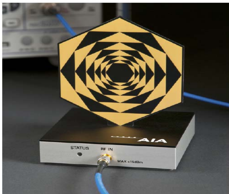
Figure 5.3-1: Audio Interference Analyzer
