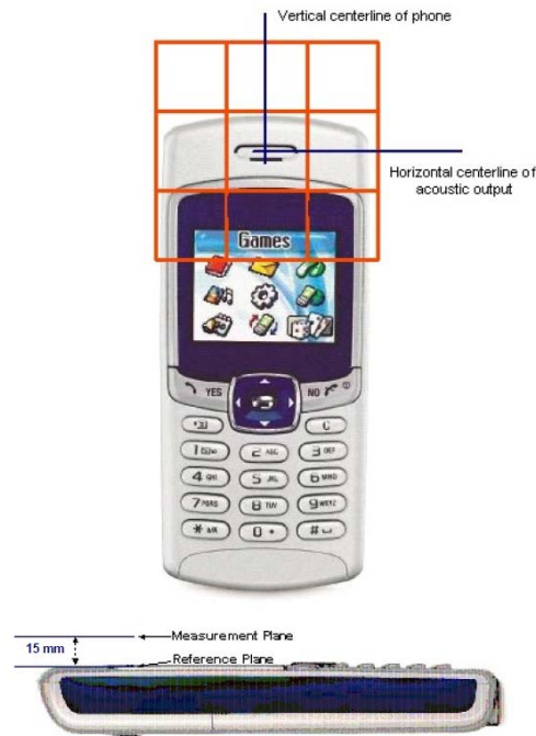
Figure 5.5-2: WD reference plane for RF emission measurement
