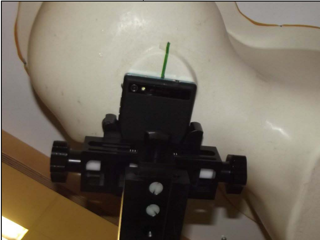
Photo 12: Test position left hand tilted 15°
