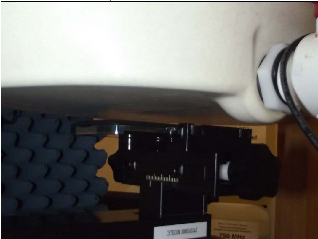
Photo 22: Test position MHS rear side with 10 mm distance
