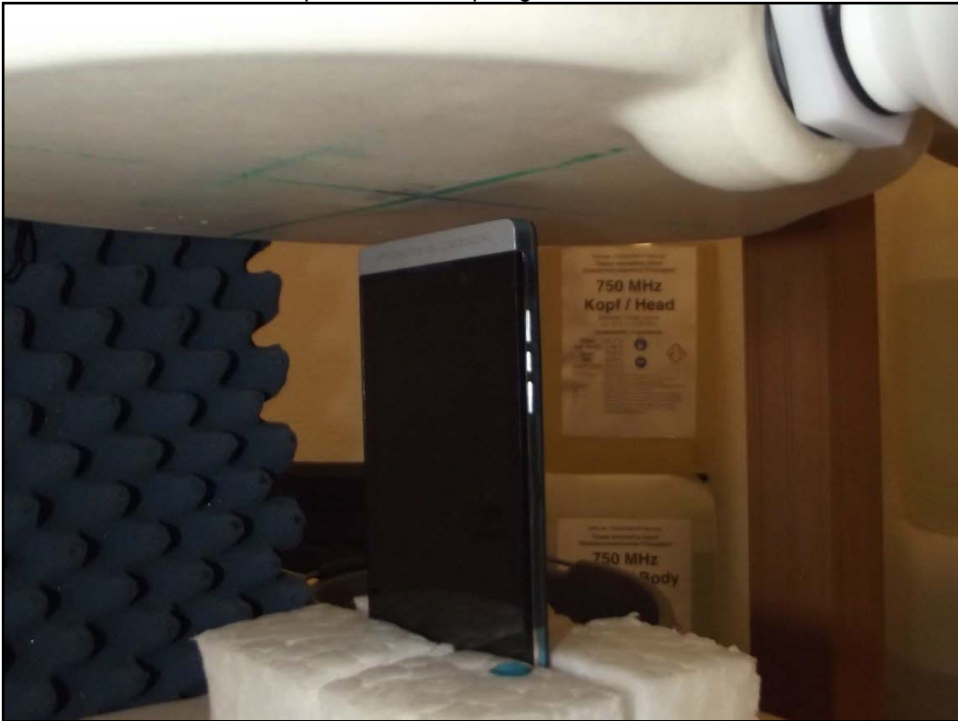
Photo 25: Test position MHS top edge side with 10 mm distance
