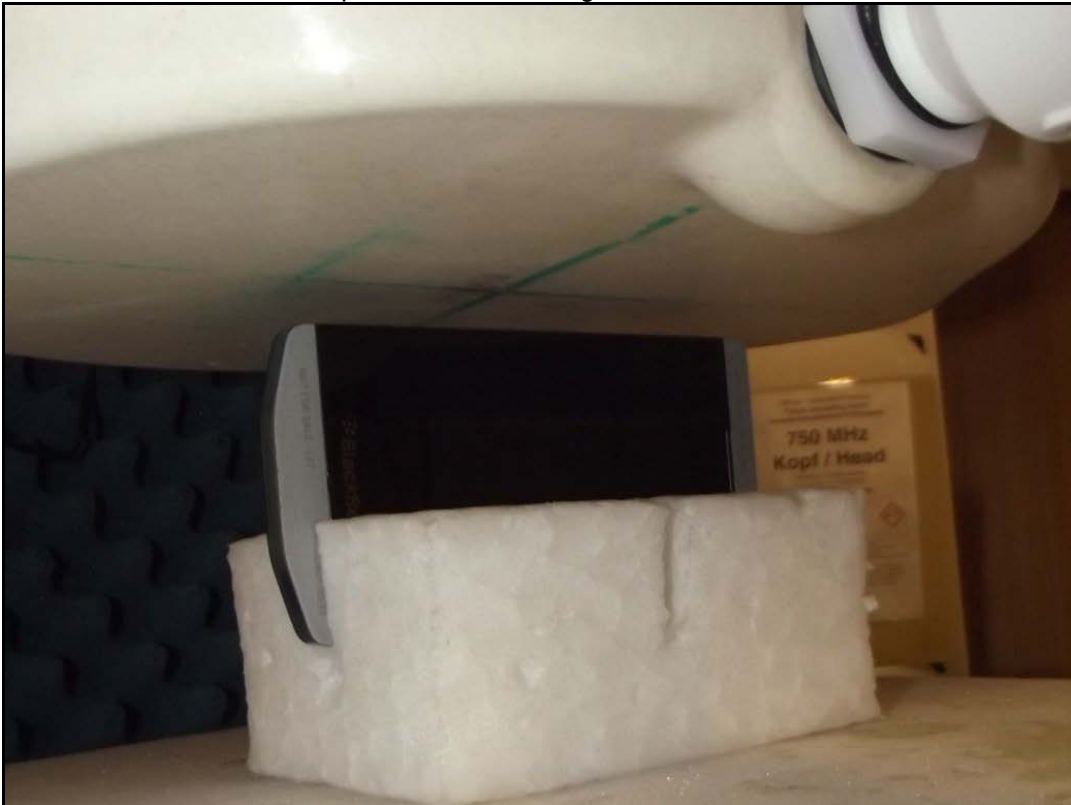
Photo 23: Test position MHS left edge side with 10 mm distance
