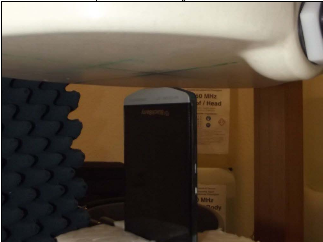
Photo 26: Test position MHS bottom edge side with 10 mm distance
