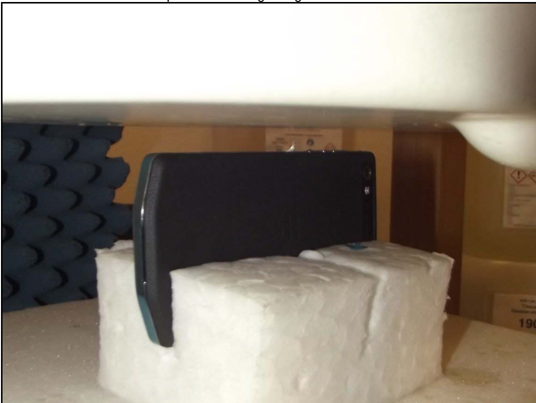
Photo 24: Test position MHS right edge side with 10 mm distance
