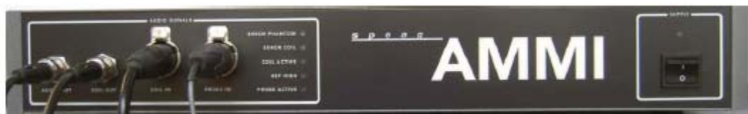
Figure 5.0-2. The Audio band Magnetic field Measuring Instrument (AMMI)
