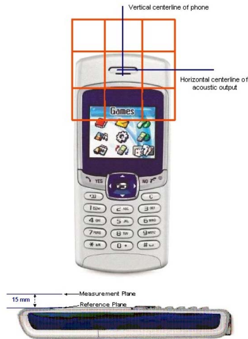
Figure 5.5-2: WD reference plane for RF emission measurement
