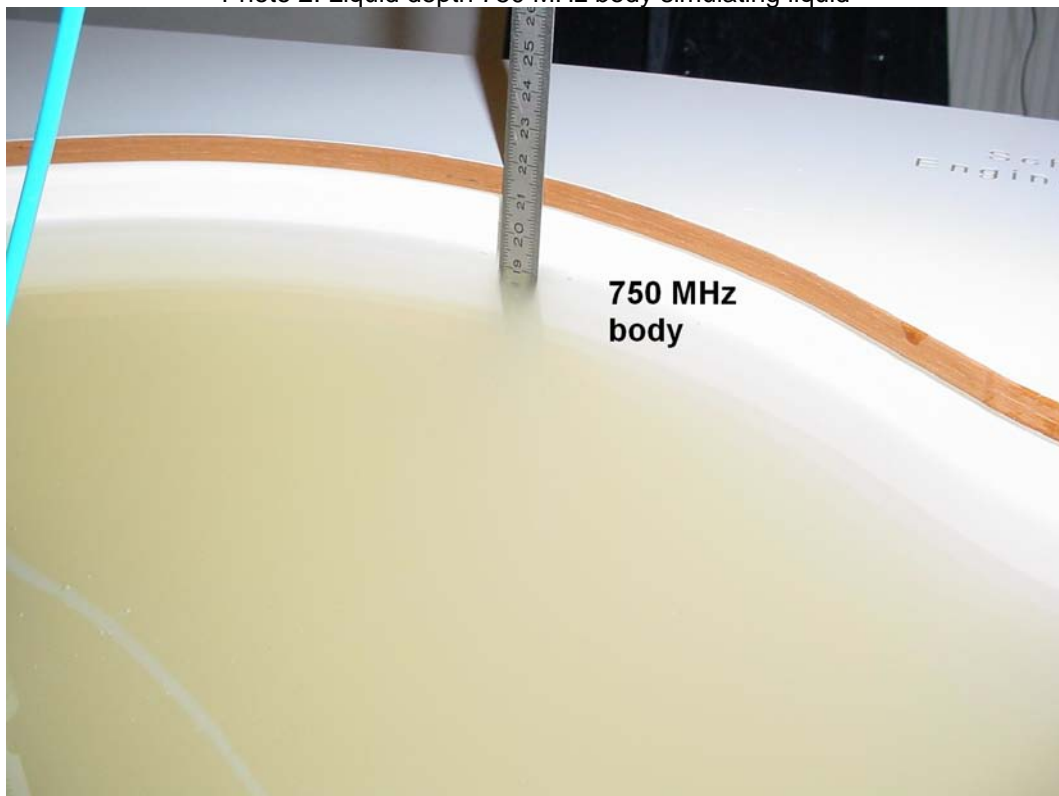
Photo 2: Liquid depth 750 MHz body simulating liquid
