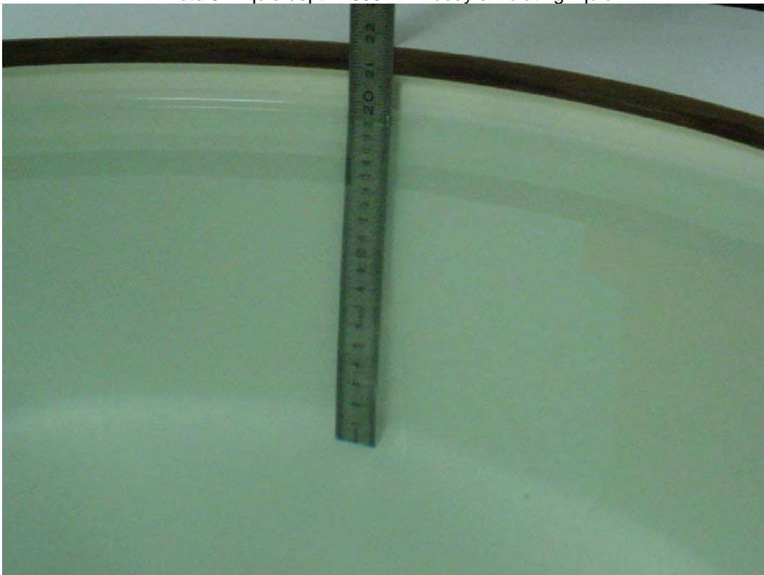
Photo 6: Liquid depth 1800 MHz body simulating liquid
