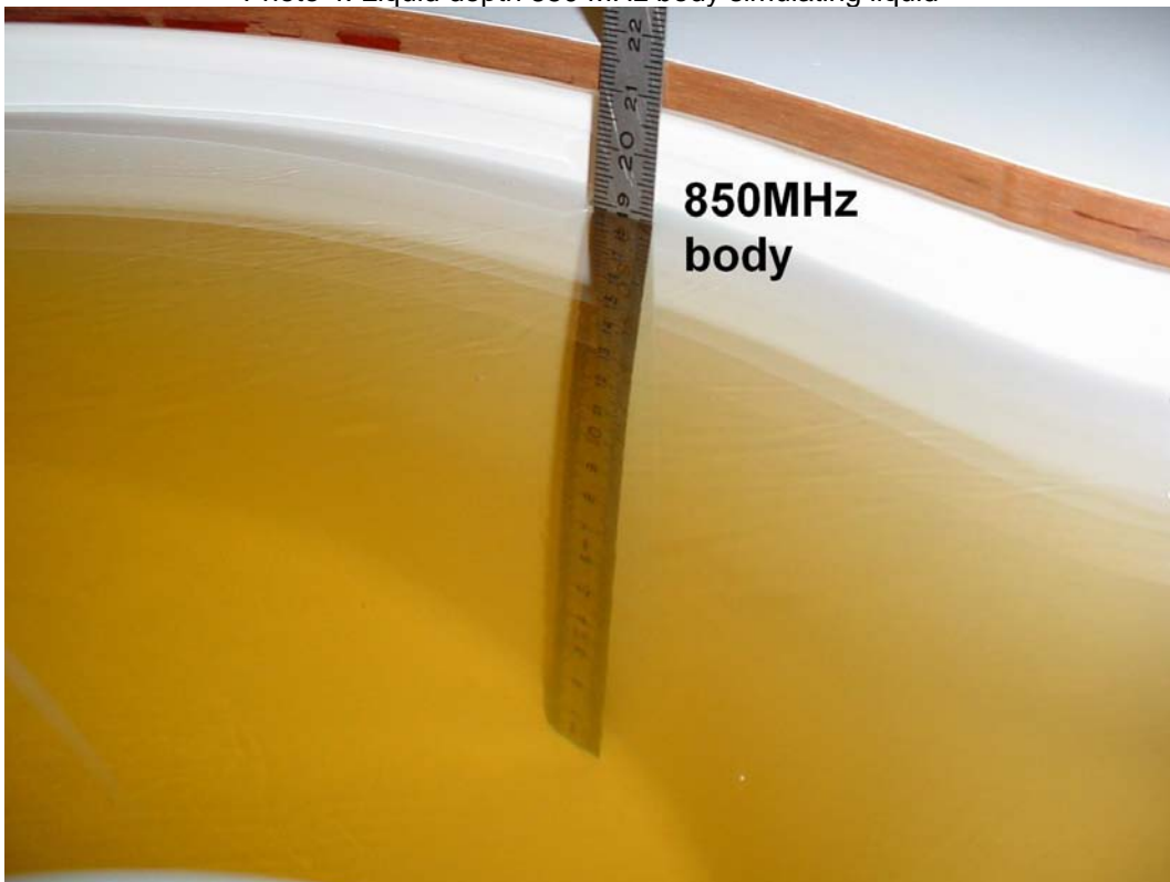
Photo 4: Liquid depth 850 MHz body simulating liquid
