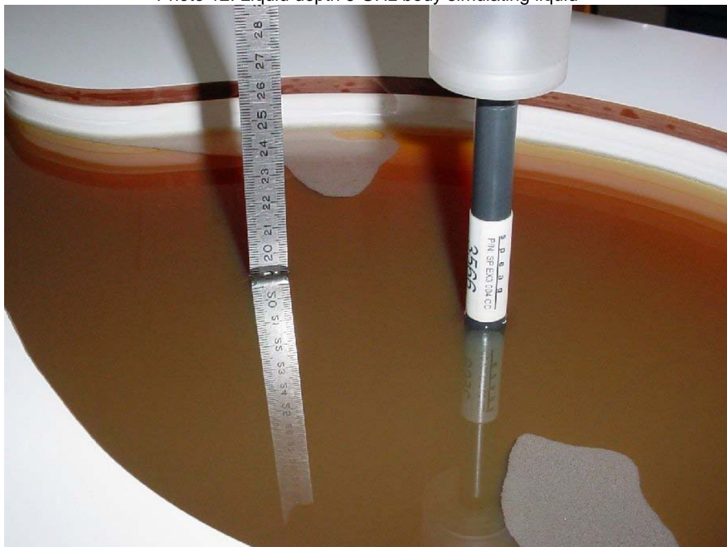
Photo 12: Liquid depth 5 GHz body simulating liquid
