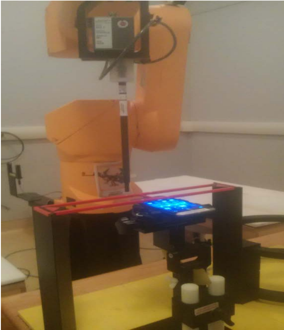
Figure C3 – HAC RF emission test setup
