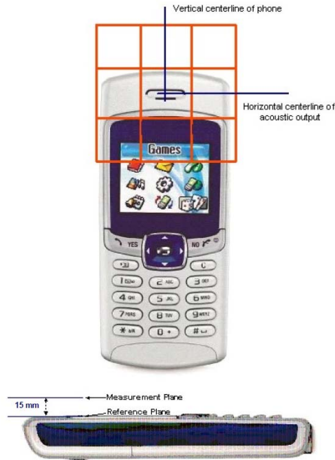
Figure 5.5-2: WD reference plane for RF emission measurement
