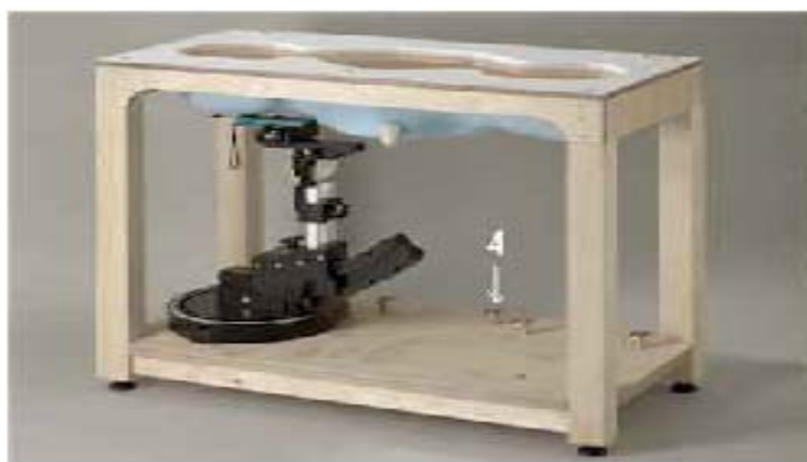
Figure 5.0-1 SAM Twin Phantom
