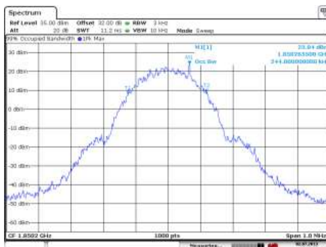
Figure 1-20a: Occupied Bandwidth, PCS1900 Low Channel in GSM mode
