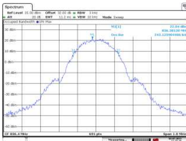
Figure 1-30a: Occupied Bandwidth, GSM850 Band, Middle Channel in EDGE mode
