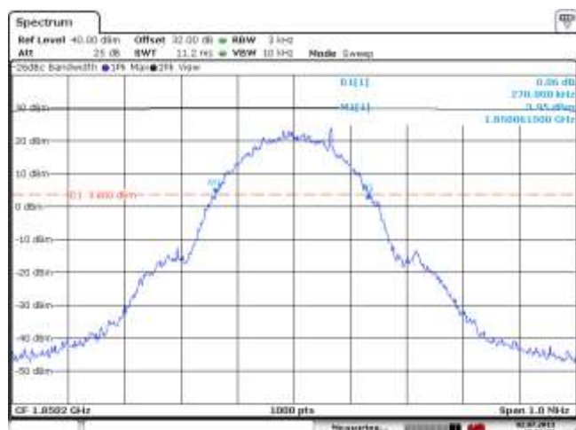
Figure 1-19a: -26dBc bandwidth, PCS1900 Low Channel in GSM mode
