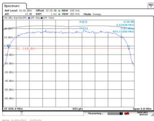
Figure 2-19a: -26 dBc Bandwidth, Band 5 Low Channel
