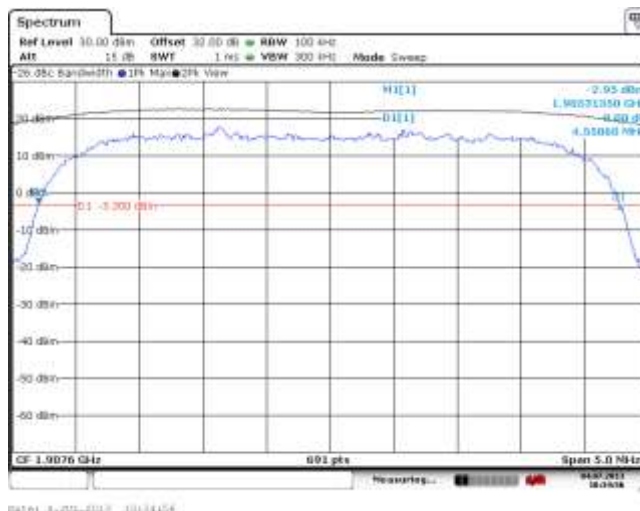
Figure 2-24a: -26 dBc Bandwidth, Band 2 High Channel
