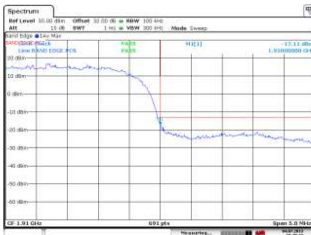
Figure 2-28a: Band 2 High Channel Mask
