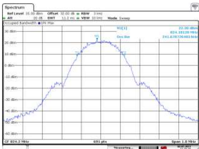
Figure 1-29a: Occupied Bandwidth, GSM850 Band, Low Channel in EDGE mode
