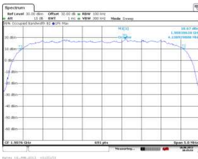
Figure 2-18a: Occupied Bandwidth, Band 2 High Channel
