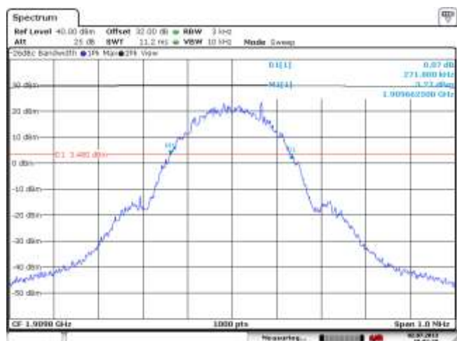
Figure 1-23a: -26dBc bandwidth, PCS1900 High Channel in GSM mode
