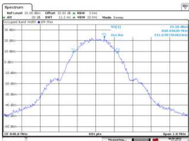
Figure 1-31a: Occupied Bandwidth, GSM850 band, High Channel in EDGE mode
