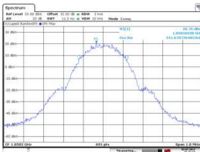
Figure 1-32a: Occupied Bandwidth, PCS1900 Band, Low Channel in EDGE mode
