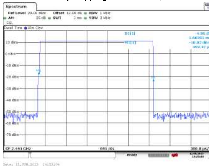
Figure 2-21: Time of Occupancy (Dwell Time) Freq. Hopping, Static PBRs, DH3
