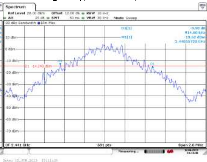
Figure 2-2: 20 dB Bandwidth Single freq., Static PBRs, DH5
