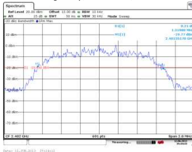
Figure 2-4: 20 dB Bandwidth Single freq., Static PBRS, 2-DH5
