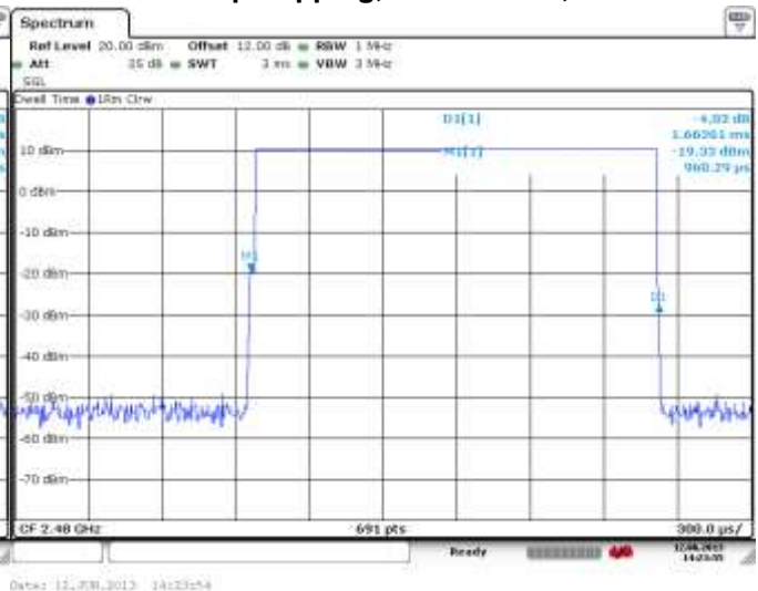
Figure 2-22: Time of Occupancy (Dwell Time) Freq. Hopping, Static PBRs, DH3
