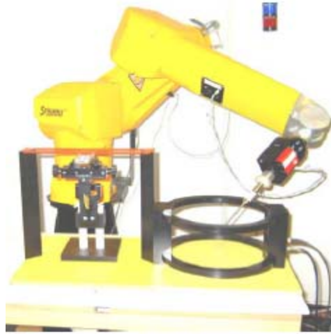
Figure 5.0-1: T-Coil set up with HAC Test Arch with Helmholtz Coil (AMCC)
