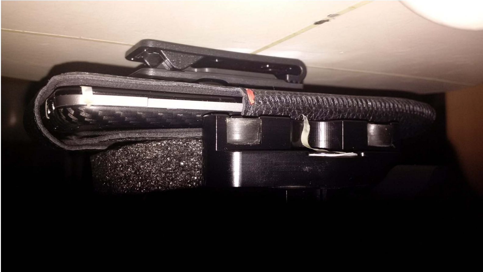
Figure E9. Body-worn configuration (Vertical Holster, front facing phantom)
