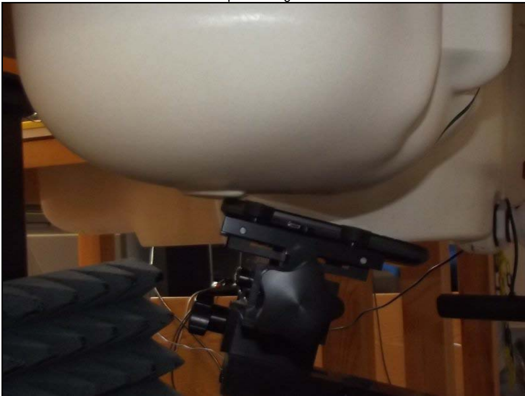
Photo 16: Test position right hand tilted 15°
