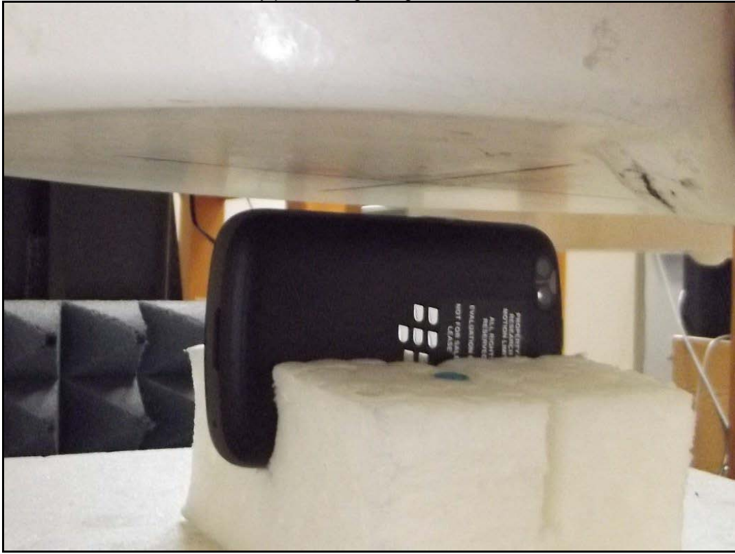
Photo 24: Test body position bottom edge side with 10 mm distance
