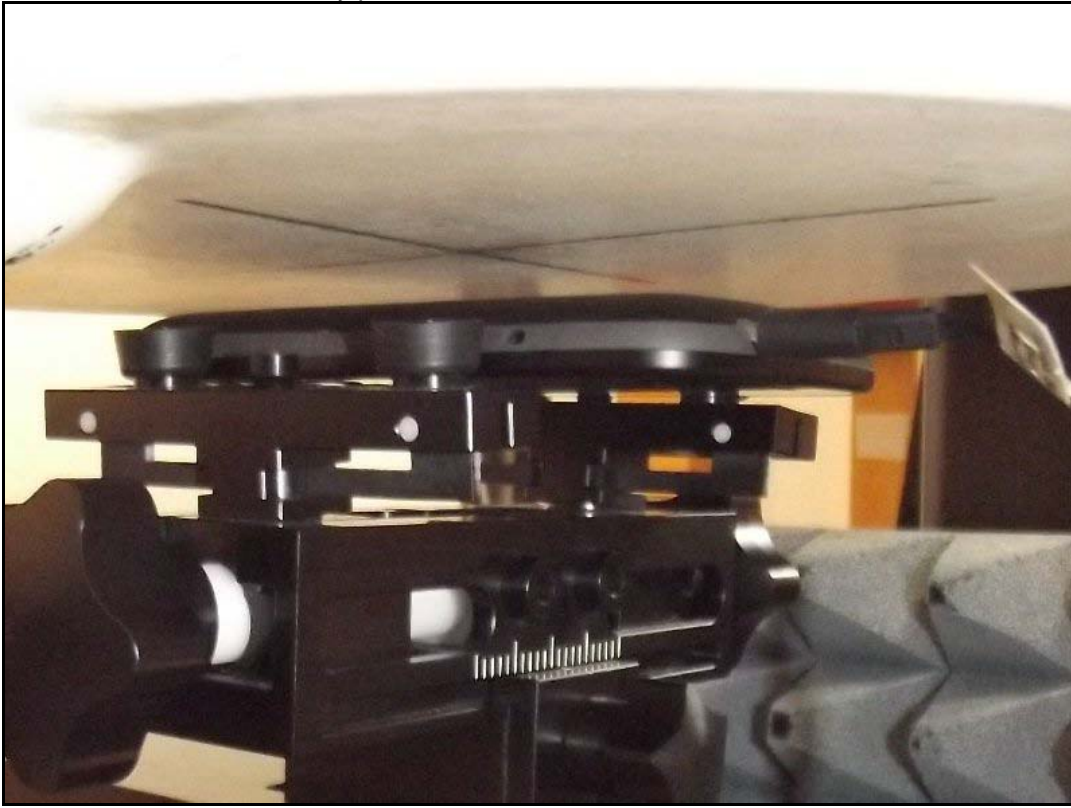
Photo 22: Test body position left edge side with 10 mm distance
