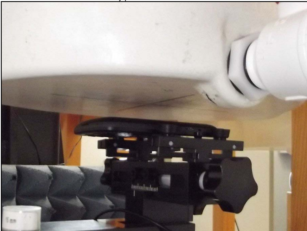
Photo 18: Test body position rear side with 15 mm distance
