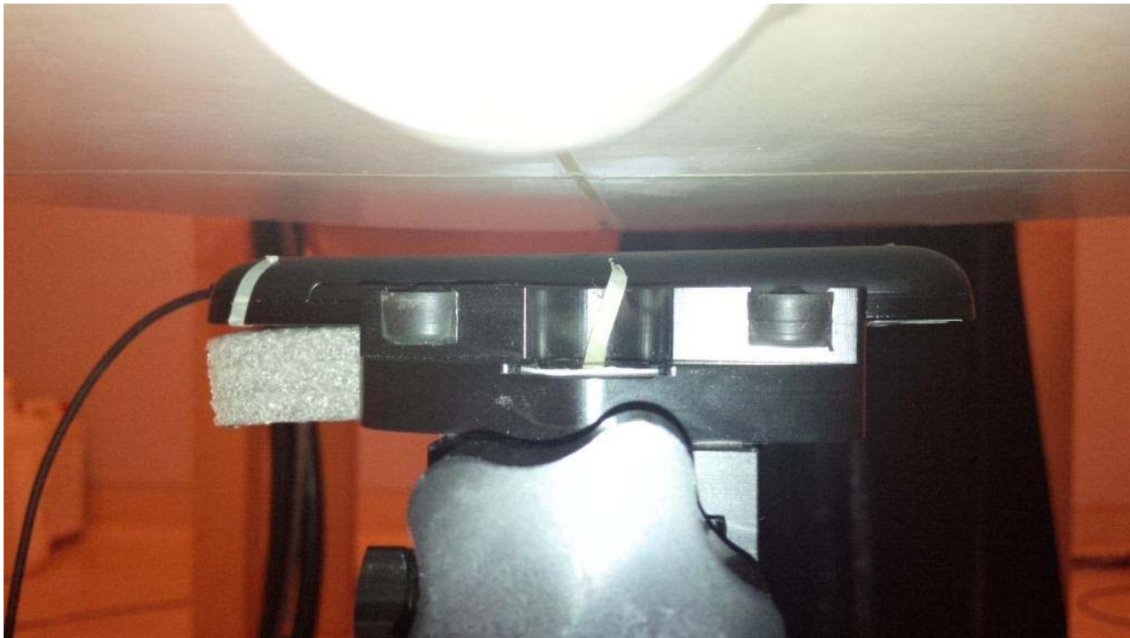
Figure E10. Body-worn configuration (No Holster, headset, back 15mm away)
