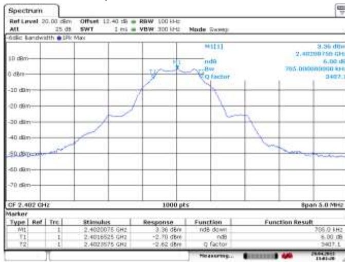
Figure 4-59: 6 dB Bandwidth LE, Channel 0
