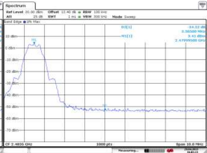
Figure 4-63: Band Edge Compliance LE, Channel 39
