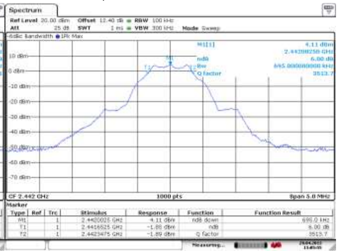
Figure 4-60: 6 dB Bandwidth LE, Channel 20
