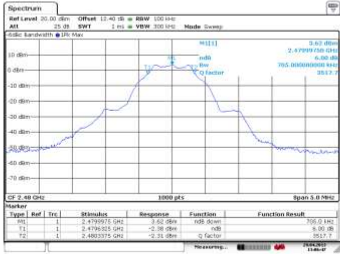
Figure 4-61: 6 dB Bandwidth LE, Channel 39
