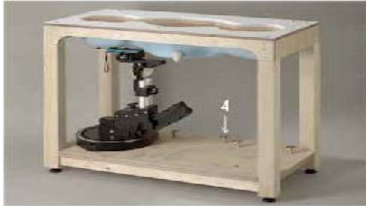
Figure 5.0-1 SAM Twin Phantom
