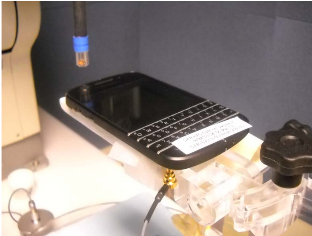
Photo 3: Transverse Probe with Wireless Device – Radial B Direction
