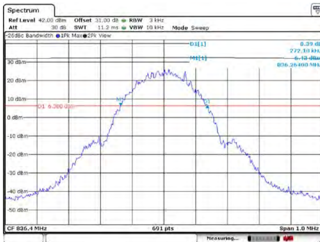
Figure 1-15a: -26dBc bandwidth, GSM850 band Middle Channel in GSM mode
