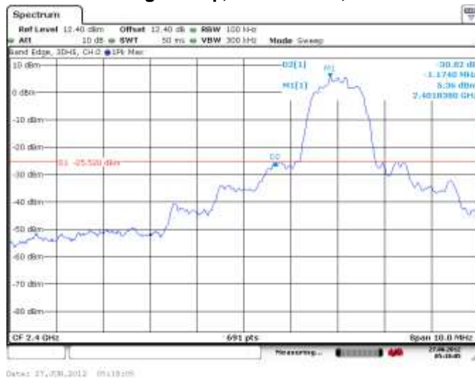
Figure 4-43: Band Edge Compliance Single Freq., Static PBRs, 3-DH5
