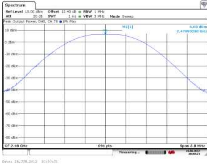
Figure 4-28: Max. Peak Conducted Output Power Single Freq., Static PBRs, DH5
