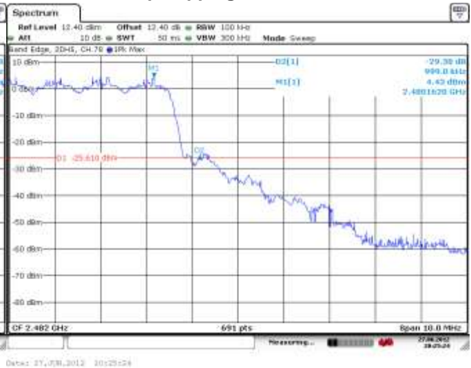
Figure 4-42: Band Edge Compliance Freq. Hopping, Static PBRs, 2-DH5
