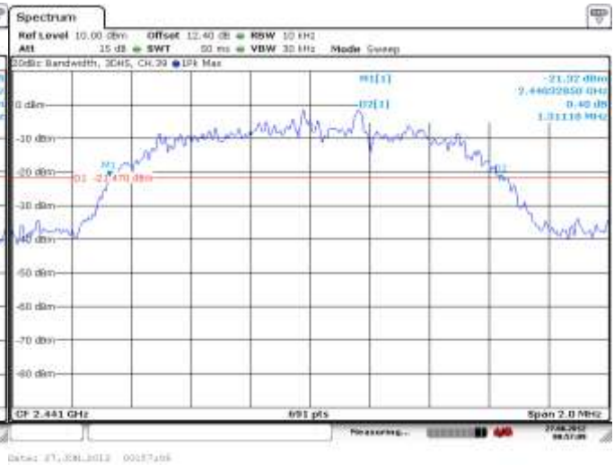
Figure 4-8: 20 dB Bandwidth Single freq., Static PBRs, 3-DH5
