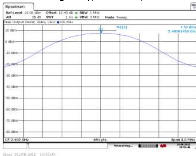
Figure 4-32: Max. Peak Conducted Output Power Single Freq., Static PBRs, 3-DH5
