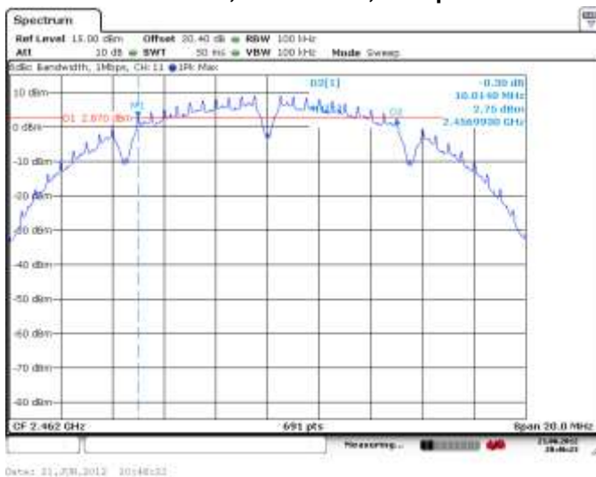
Figure 5-3: 6 dB Bandwidth 802.11b, Channel 11, 1 Mbps
