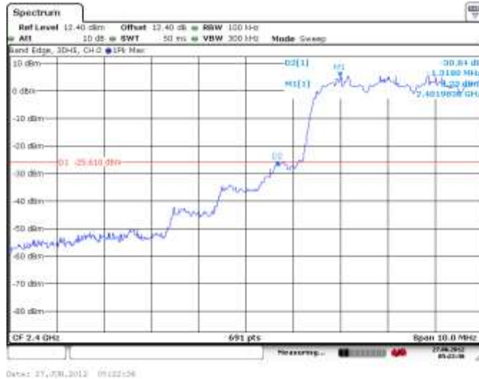
Figure 4-45: Band Edge Compliance Freq. Hopping, Static PBRs, 3-DH5
