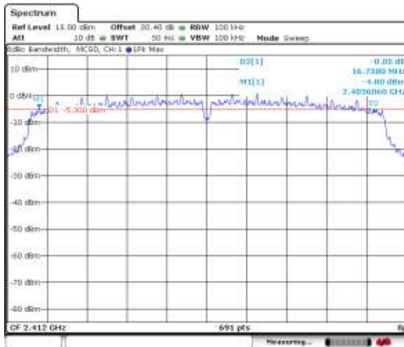
Figure 5-7: 6 dB Bandwidth 802.11n, Channel 1, MCS 0
