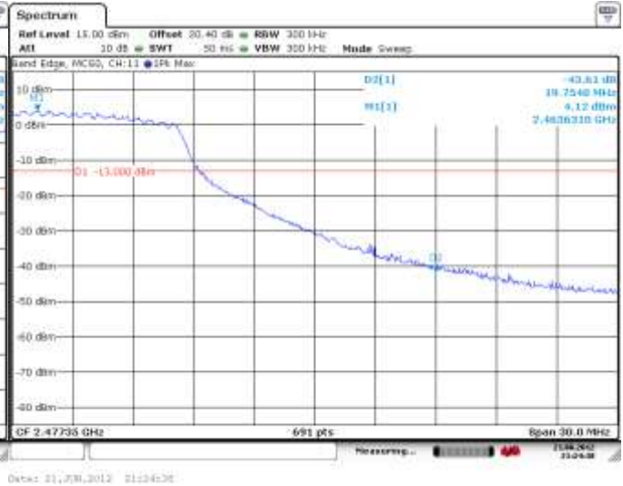
Figure 5-15: Band Edge Compliance 802.11n, Channel 11, MCS 0
