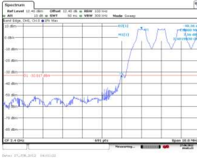
Figure 4-37: Band Edge Compliance Freq. Hopping, Static PBRs, DH5
