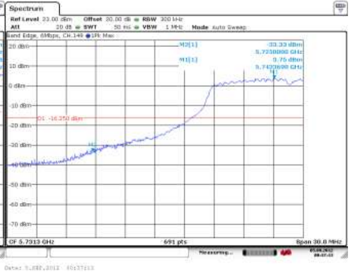
Figure 6-21: Band Edge Compliance 802.11a, Channel 149, 6 Mbps
