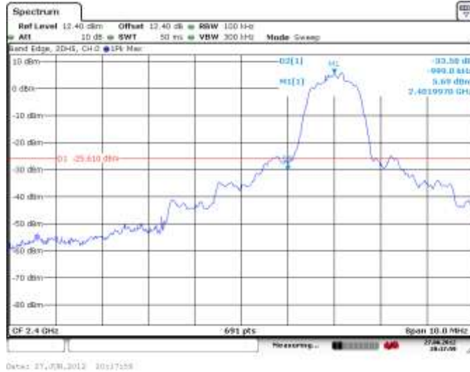
Figure 4-39: Band Edge Compliance Single Freq., Static PBRs, 2-DH5
