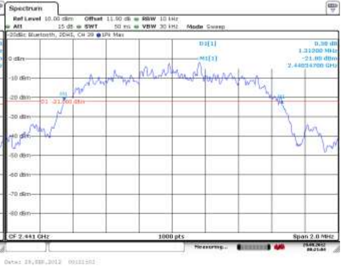
Figure 4-5: 20 dB Bandwidth Single freq., Static PBRs, 2-DH5
