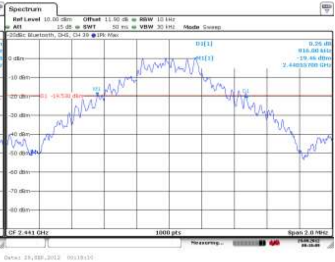
Figure 4-2: 20 dB Bandwidth Single freq., Static PBRs, DH5
