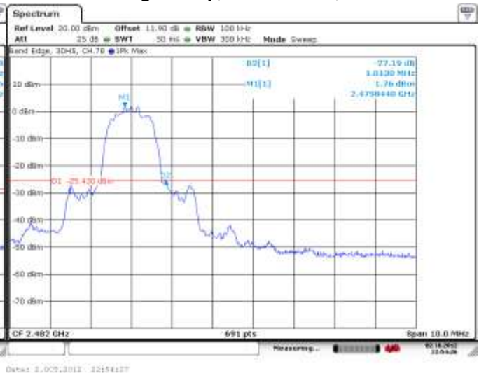
Figure 4-44: Band Edge Compliance Single Freq., Static PBRs, 3-DH5
