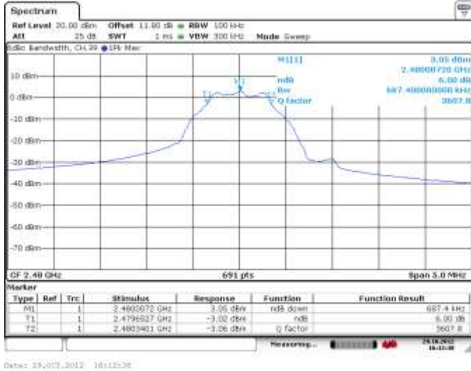
Figure 4-61: 6 dB Bandwidth LE, Channel 39
