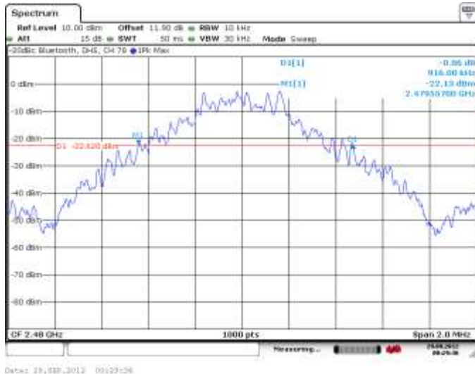
Figure 4-3: 20 dB Bandwidth Single freq., Static PBRs, DH5
