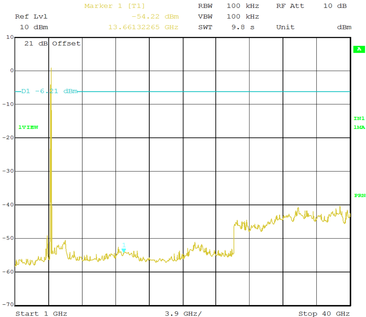
Figure 6-47a: Spurious RF Conducted Emissions, 802.11n Channel 44, 6 Mbps
