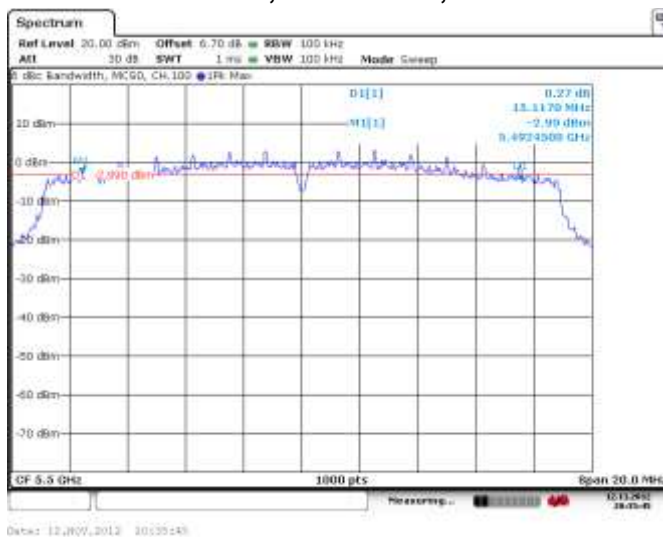
Figure 6-19: 6 dB Bandwidth 802.11n, Channel 100, MCS 0
