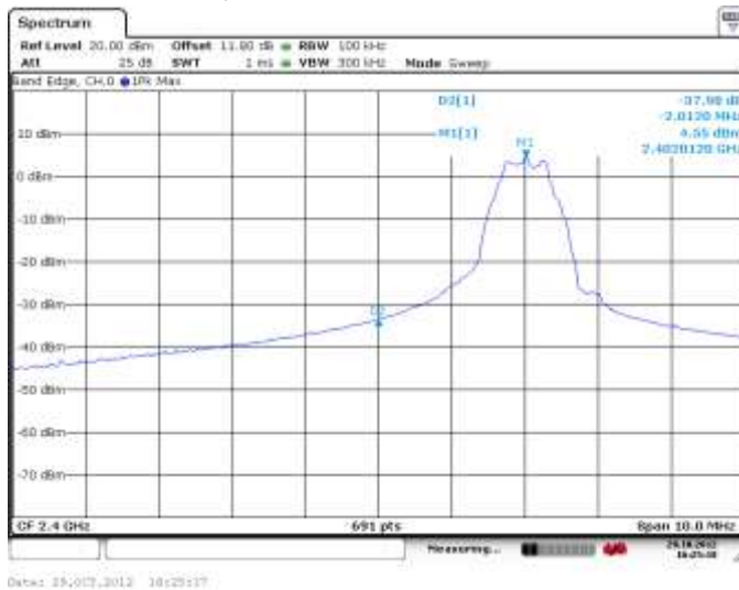
Figure 4-62: Band Edge Compliance LE, Channel 0
