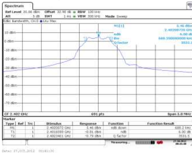
Figure 4-59: 6 dB Bandwidth LE, Channel 0
