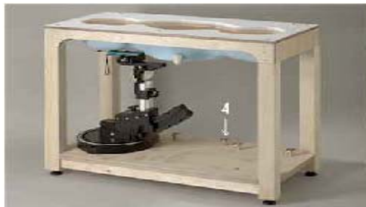
Figure 5.0.1. SAM Twin Phantom
