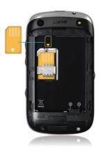
Slide the SIM card into the slot.
