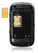
Slide the SIM card into the slot.
