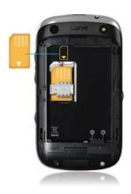
Slide the SIM card into the slot.
