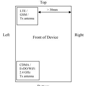
Bottom Figure 1.8.4-1 Identification of all sides for SAR Testing
