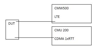
Figure 1.10.1-1 SVLTE Conducted Power Test Setup Diagram
