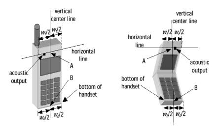
Figure 8.2.1-1 Handset vertical and horizontal reference lines – fixed case
