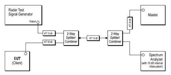
A spectrum analyzer is used as a monitor to verify that the EUT has vacated the Channel within the Channel Closing Transimission Time and Channel Move Time, and does not transmit on a Channel during the Non-Occupancy Period after the detection and Channel Move. It is also used to monitor EUT transmissions during the Channel Availability Check Time.
