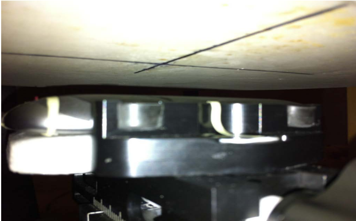
Figure E6. Body-worn configuration (No Holster, back side 15mm away)
