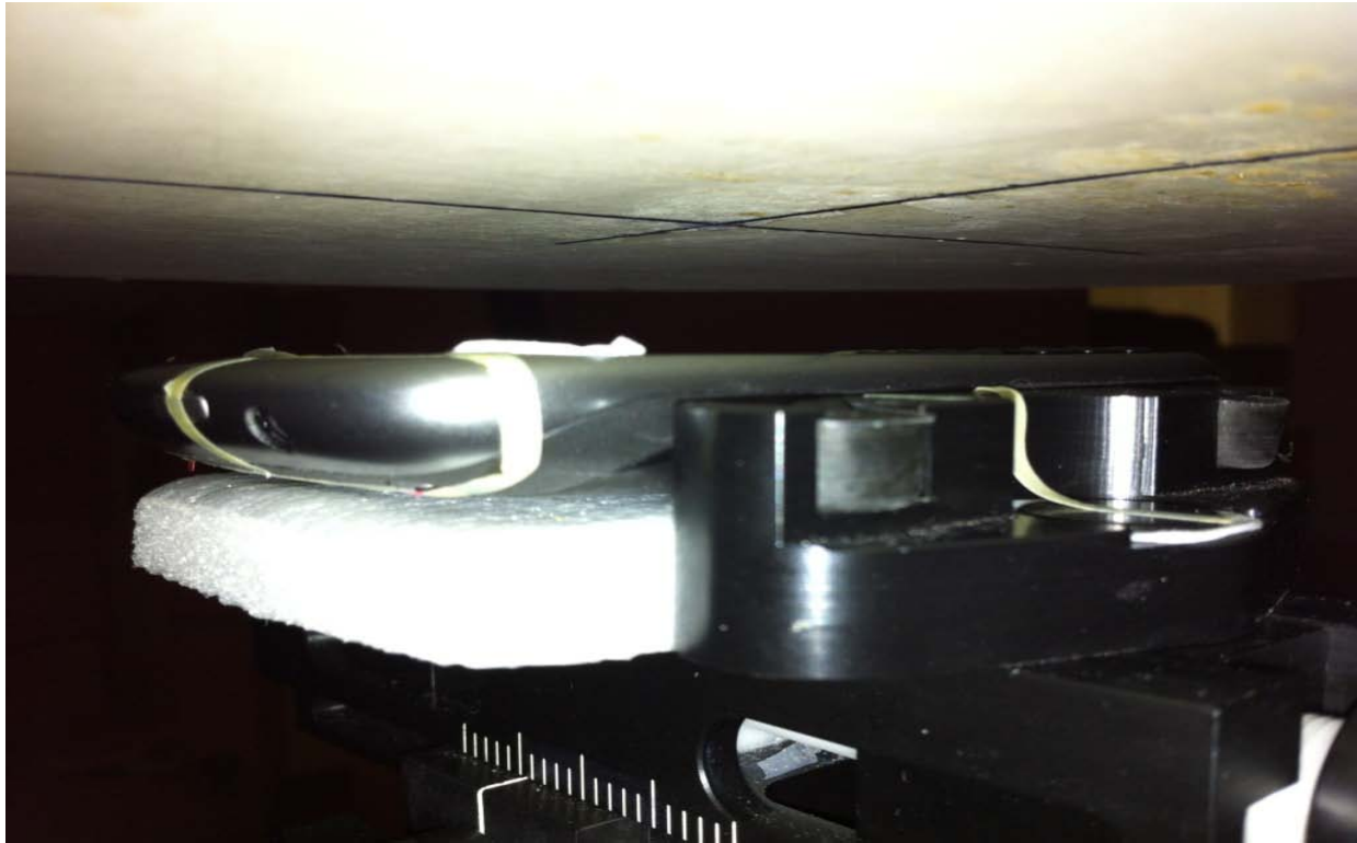
Figure E7. Body-worn configuration (No Holster, front side 15mm away)
