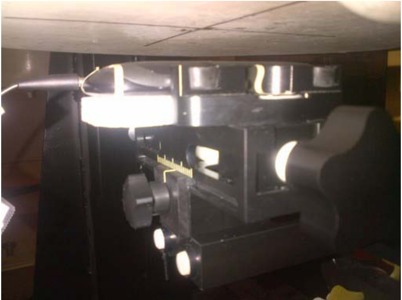
Figure E9. Body-worn configuration (No Holster, headset, back side 15mm away)
