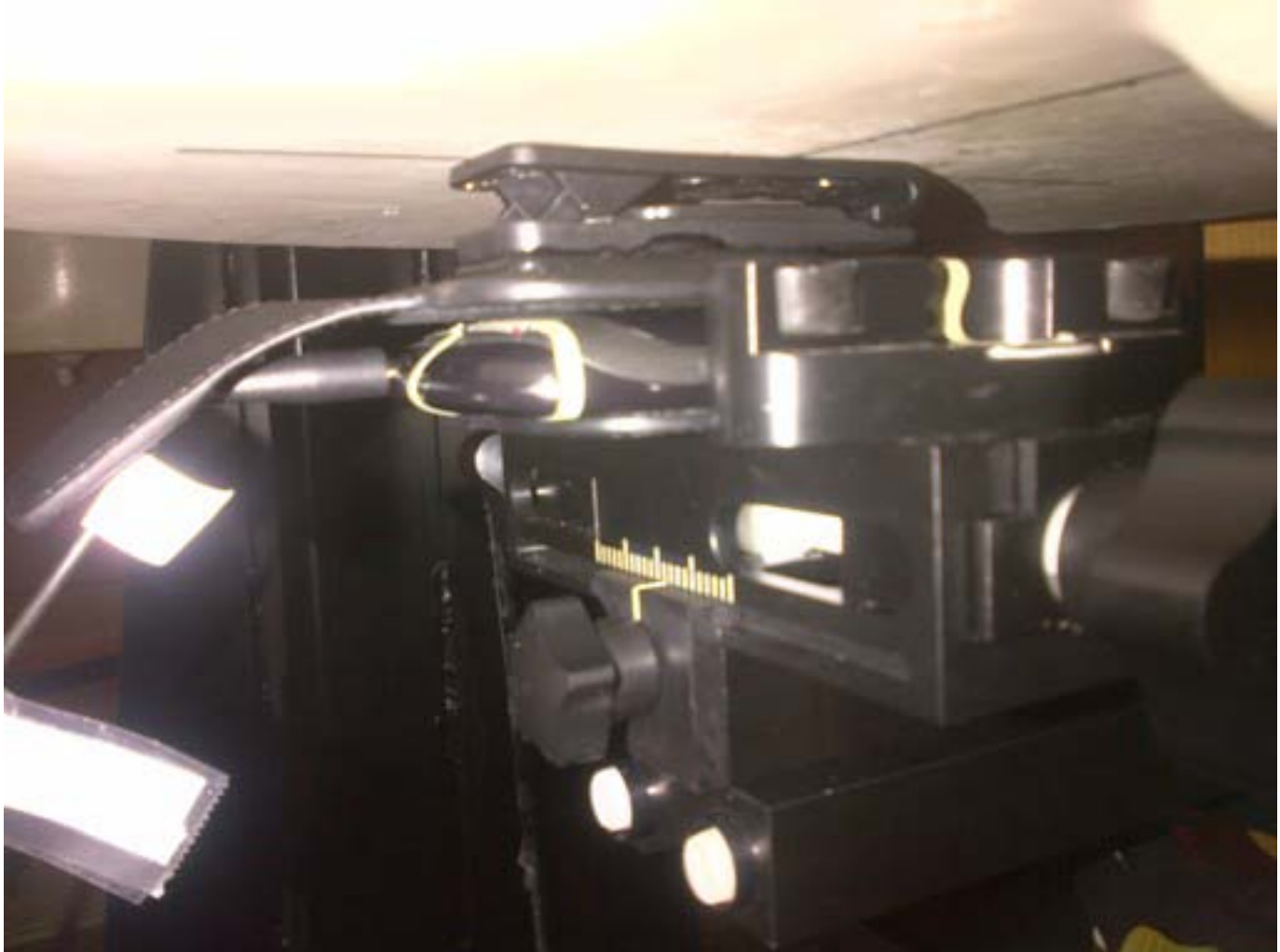
Figure E10. Body-worn configuration (Vertical Holster, headset, back side)
