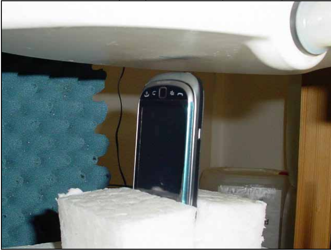
Photo 16: Test body worn position top side (10 mm distance)
