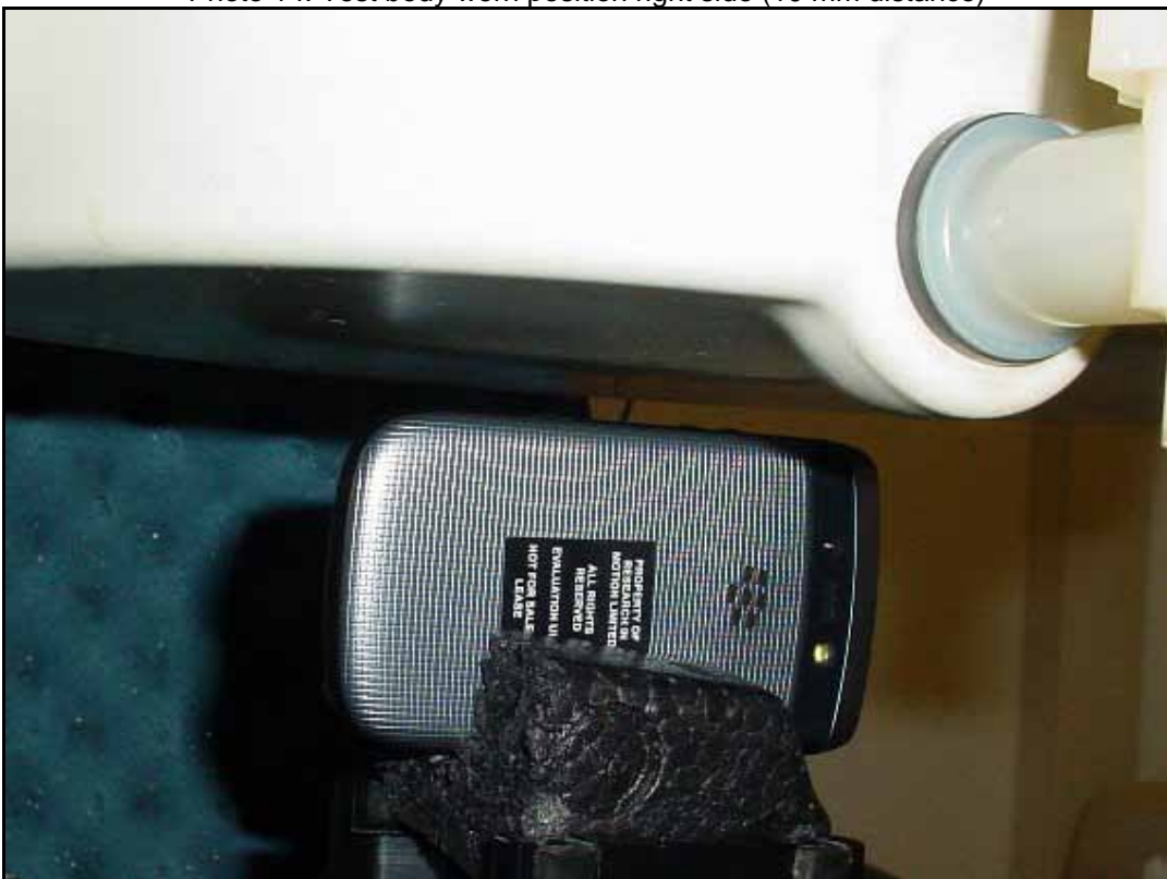
Photo 14: Test body worn position right side (10 mm distance)
