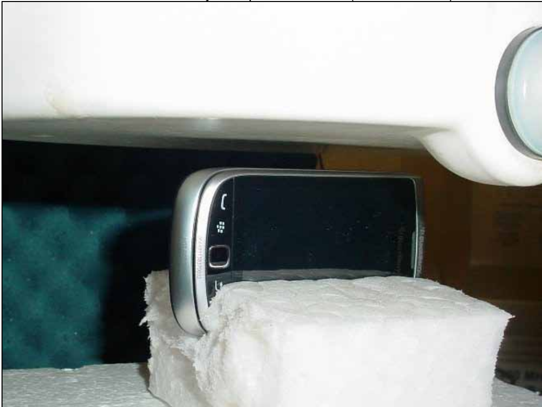
Photo 14: Test body worn position right side (10 mm distance)
